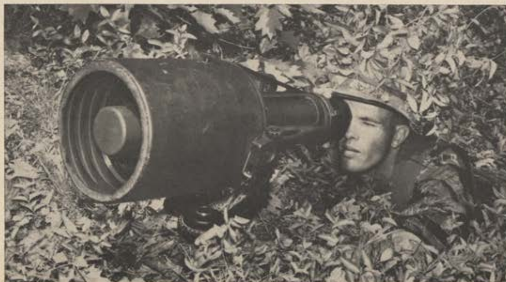
Largest of the recently declassified devices in use in Vietnam is the Night Observation Device, Medium-Range, at left. It has a range of 1,000 to 1,200 meters and is intended primarily for use on aircraft, ground vehicles, or in fixed positions.
