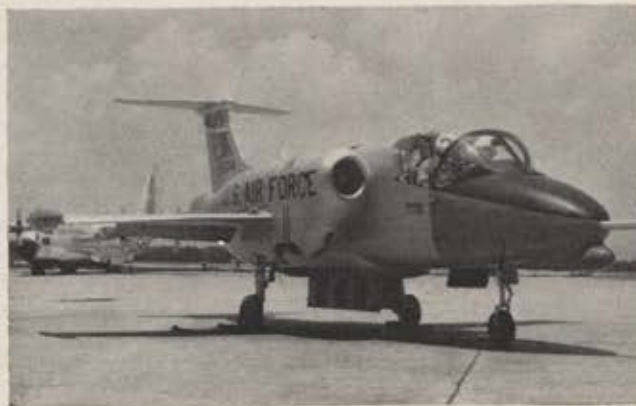
Originally built for US Army, Hummingbird has been modified for Air Force tests at Lockheed's "Possum Works" in Marietta. Note air inlets for four direct-lift engines in upper fuselage. Plane will be used in developing control characteristics for future Air Force VTOL fighter projects.
