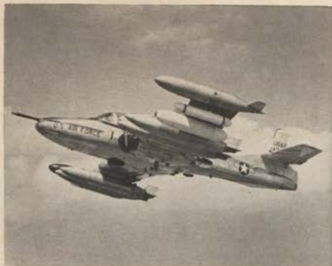
Cessna A-37Bs are now coming off assembly line at Wichita, Kan. While A-37A, which has logged more than 10,000 combat sorties in Vietnam, was modified from T-37 trainer, A-37B is entirely new plane, incorporating aerial refueling, more powerful engine, improved fire-control system, and stronger airframe stressed for 6 Gs, vs. 5 Gs in A-37A.
