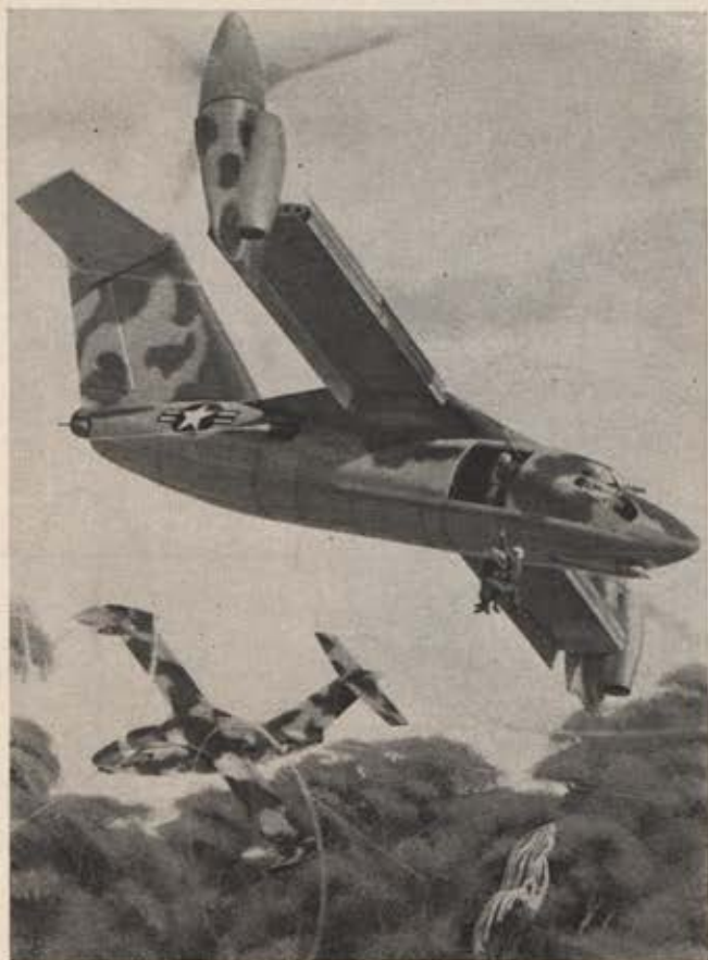
Tilt-rotor principle varies from stowed-rotor approach insofar as the rotor functions as a propeller during cruise. Stowed rotor offers greater cruise efficiency than tilting and tilt-rotor methods, but is more complex and expensive.
