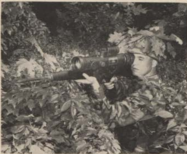
Smallest of the new family of night-vision devices is the Starlight Scope shown above attached to a carbine. This equipment was developed by the Army's Combat Surveillance, Night Vision and Target Acquisition Laboratories, at Fort Belvoir, Va., which are directed by Dr. R. S. Wiseman.
