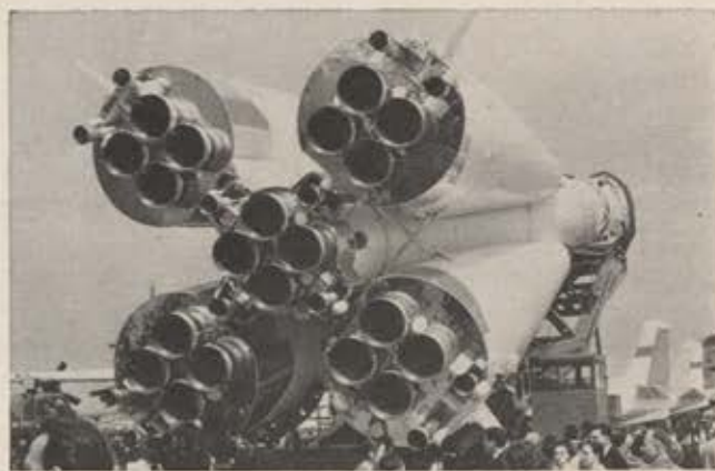
An early product of the "orderly, persistent, well-planned" Soviet space program was Vostok booster, shown in rear view. One such rocket orbited Yuri Gagarin in first Vostok.
