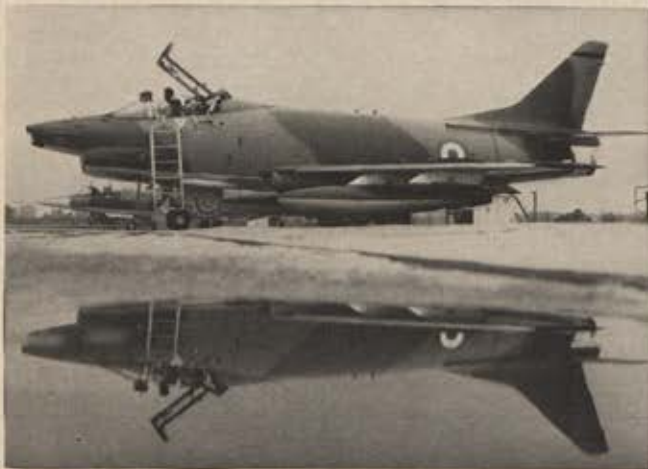
Prototype of Fiat G.91Y lightweight fighter-bomber-reconnaissance aircraft being built for Italian Air Force was displayed at 3d International Aeronautics and Space Show in Turin, Italy, early in June. Single-seater is powered by two GE J85-13 turbojets of 4,080 pounds thrust each.
