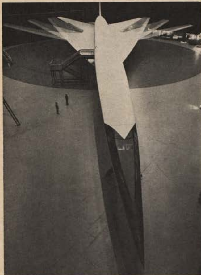
Variable-sweep wing feature of the SST is shown in triple-exposure view of SST mockup in Seattle: wings positioned for takeoff (fully extended), for subsonic cruise (intermediate position), and for supersonic cruise (folded back).
