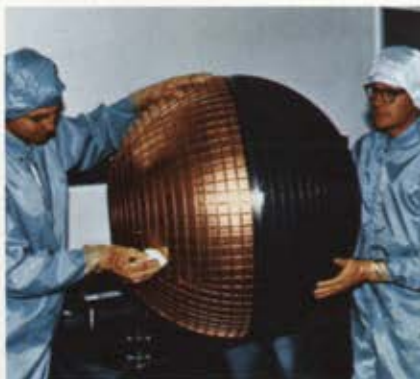
This liquid hydrogen tank, designed and fabricated by Beech, incorporates advanced thermal protection systems recently developed by Beech.
