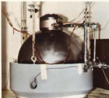
Beech designed and fabricated tank for liquid oxygen undergoes testing. Two of these provide a two-week supply to the Apollo Command module.
