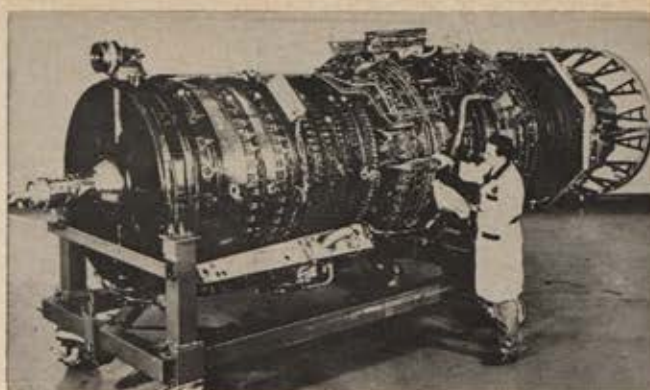
General Electric GE4 afterburning turbojet, above, being developed for SST, is very similar to the GE YJ93, which powers the XB-70. General Electric says its design objective was to achieve simplicity. One of the most advanced jets ever built, its turbine-inlet temperature is around 2,400° F.
