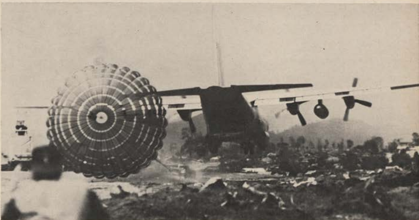
Using the Low Altitude Parachute Extraction System (LAPES), an Air Force C-130 Hercules crew delivers a load of supplies to the US Army's 1st Cavalry Division (Airmobile) at An Khe. With LAPES, platform-mounted loads are pulled from the rear of a transport plane at an altitude of about five feet. System is designed for resupply in narrow drop zones.
