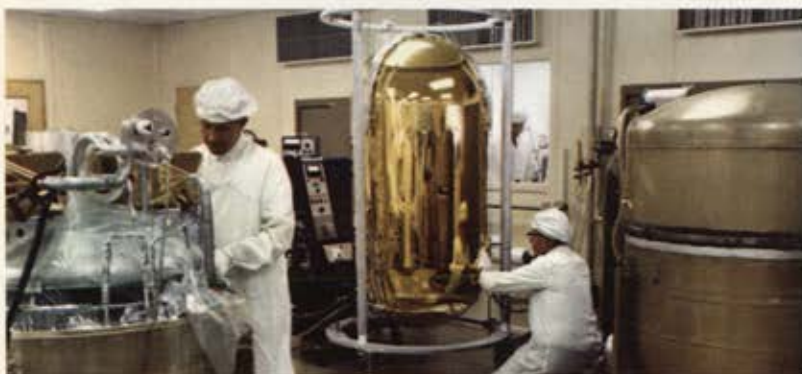
These high pressure Dewars to contain supercritical hydrogen and supercritical oxygen for ground use were designed and manufactured at Boulder. These Dewars will work at 250 and 1000-pound pressures, respectively, and are an example of the cryogenics-associated projects that Beech carries through from design to completion.
