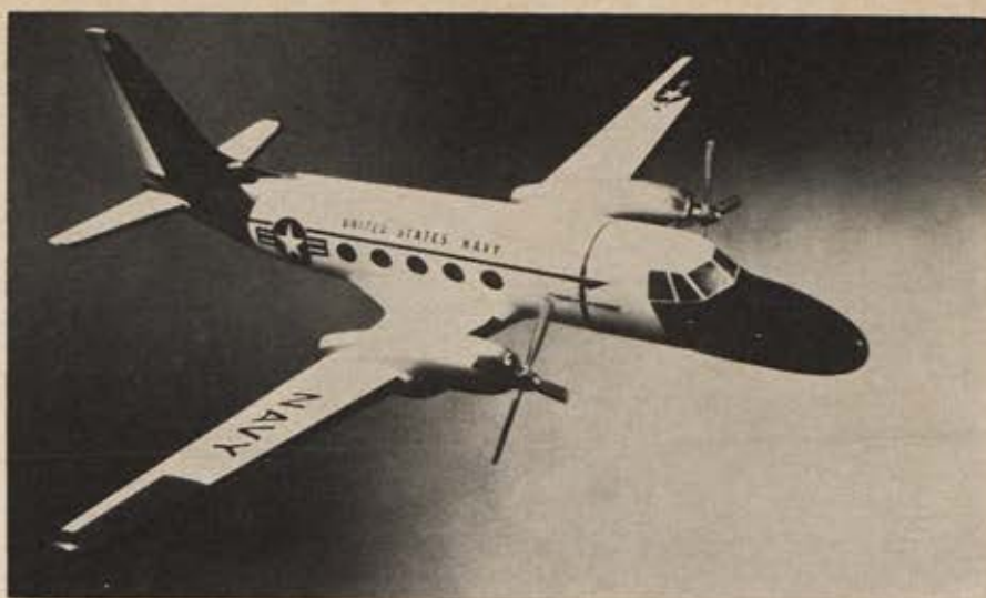
Navy is buying nine Grumman Gulfstream I turboprop light transports for use in training crews for Grumman A-6A Intruder. Designated TC-4C, plane is fitted with Intruder radome nose housing search and track radar antennas. Cabin contains separate A-6A avionics system with cockpit for student pilot and bombardier/navigator, and instrument readout consoles for four additional students.
