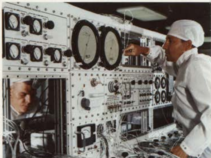
Apollo Bench Maintenance Equipment. Systems to test and functionally certify airborne components and modules of the Apollo spacecraft's Beech-built Cryogenic Storage Subsystem are built by the Boulder division. The first of these intricate equipments is installed at Cape Kennedy now.
