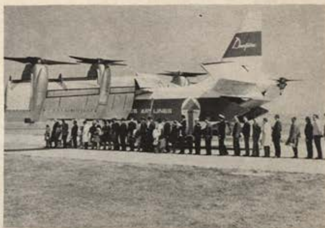
Quick "cardboard" conversion of LTV's triservice XC-142A experimental military tilt-wing V/STOL results in "Downtown," the company's idea for a forty-four-passenger commercial air commuter, which can function in the VTOL, the STOL, or the conventional mode with equal ease.
