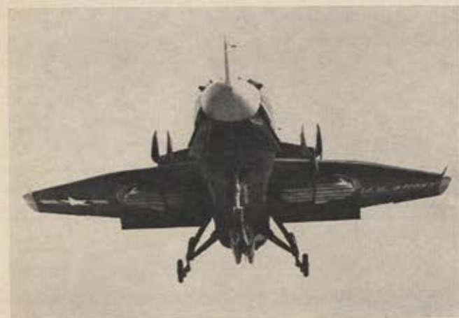
Challenging and difficult V/STOL technique known as fan-in-wing is employed by XV-5A research vehicle. Photo shows open louvers underneath the fan at bottom of wing, open butterfly fan covers atop wing, and open pitch fan entry louvers and exit control doors in nose.
