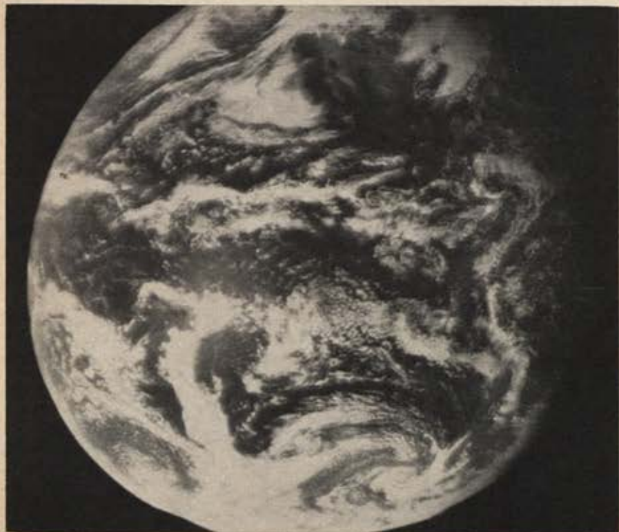
This photo of almost the entire disc of the earth was taken on December 9 from an altitude of 23,000 miles over the Pacific by the spin scan cloud camera aboard NASA's Applications Technology Satellite (ATS-1). The relatively cloud-free area in the upper center exposes Central America and southern portions of North America. This type of picture can be made once every twenty minutes.
