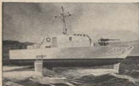
PGH (Patrol Gunboat-Hydrofoil), designed and being built by Boeing, will be first of its kind for U.S. Navy. Propulsion is by water-jet engine.
