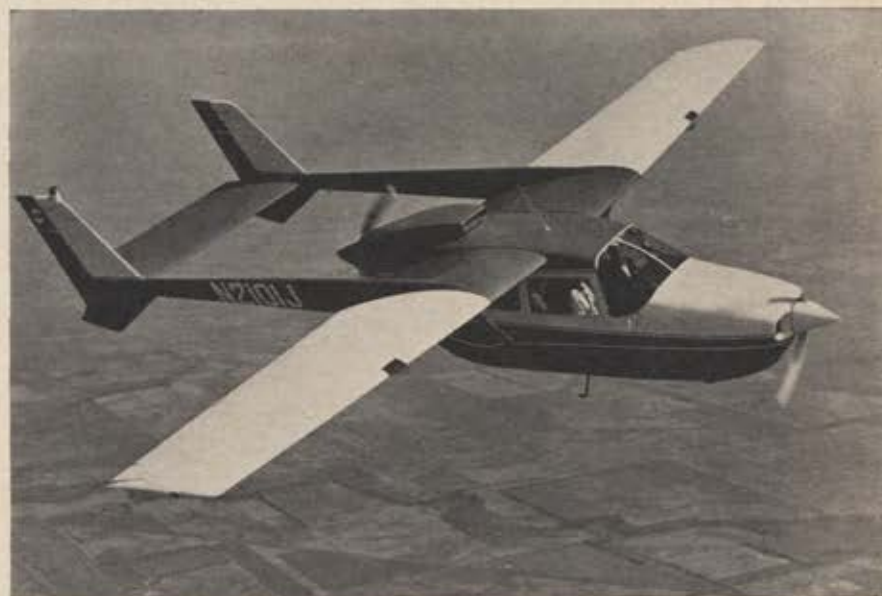
Selected by USAF to replace the O-1 Bird Dog for Forward Air Controllers in Vietnam is the Cessna 337 Super Skymaster. It is powered by two 210-horsepower Continental IO-360 engines, cruises at 190 mph, climbs 1,300 feet per minute, and can stay aloft five hours. With maximum gross takeoff weight of 4,200 pounds, it can carry pilot, observer, and a modest weapons payload.
