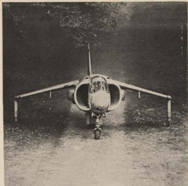
This small clearing makes an adequate airstrip for the P.1127, big enough for a short takeoff roll as well as vertical launch. With plane's easy maintainability, this location could readily hide essential ground equipment.
