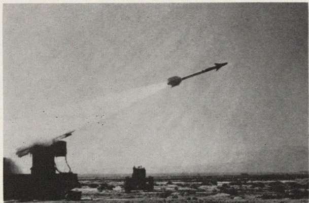
First firing tests of U.S. Army's Chaparral surface-to-air antiaircraft missile system were conducted recently at the Naval Ordnance Test Station, China Lake, California. The Chaparral, a modification of the Sidewinder air-to-air missile, is mounted on an M548 self-propelled vehicle of the U.S. Army.
