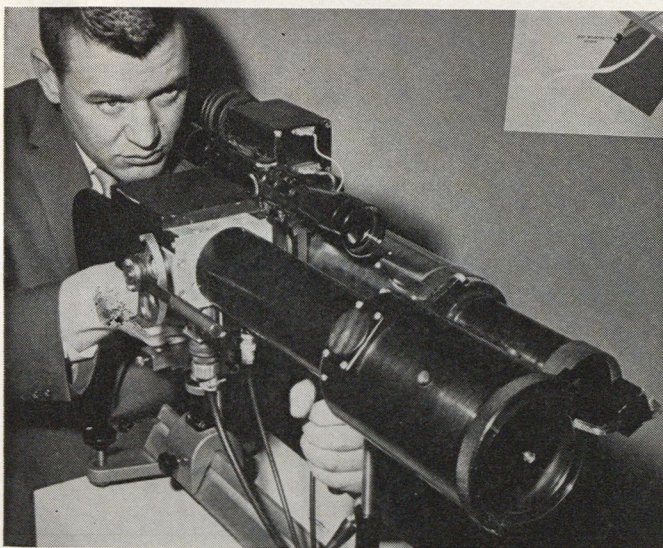
Portable "laser" ranger, developed at General Electric Company's electronics laboratory in Syracuse, New York, may be employed as a surveying tool. The range-finder weighs less than 30 pounds (13.5 kg) and has an accuracy of plus or minus 1 foot (30.48 cm) at distances up to 50,000 feet (15,200 m).
