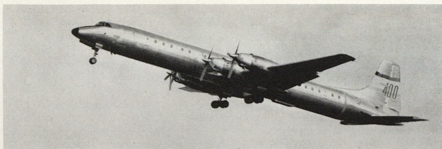
Canadair will deliver 2 of its new "400" transports to Loftleidir/Icelandic Airlines in March. The 400, or CL-44J, a stretched version of the CL-44D4 passenger/cargo aircraft, is 182 inches (462 cm) longer than the 44D and carries 189 passengers, an increase of 29 over the CL-44D. Here it departs from Cartierville Airport on an early test flight.
