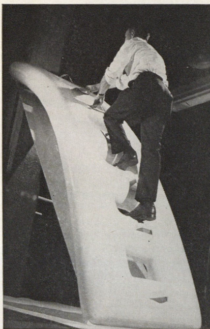
To inspect interior of hydrogen tanks in Saturn S-1VB stage, accessible only from 18-inch (45.7 mm) aperture, Goodyear's Aviation Products Division fabricated this inflatable ladder. Deflated, it rolls into 12-inch (30.5 mm) bundle. Inflated with nitrogen, it extends to 11 feet (335 cm), and is strong enough to support 2 men.
