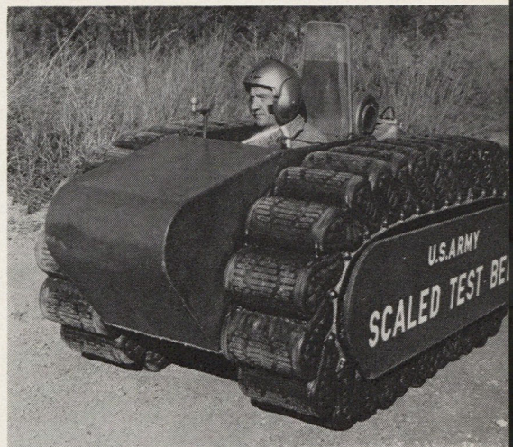
U.S. Army's PATA (pneumatic all-terrain amphibian) vehicle, shown on page 43 of the January issue, was preceded by this one-man scale model built and tested by its designer, Ling-Temco-Vought Co.
