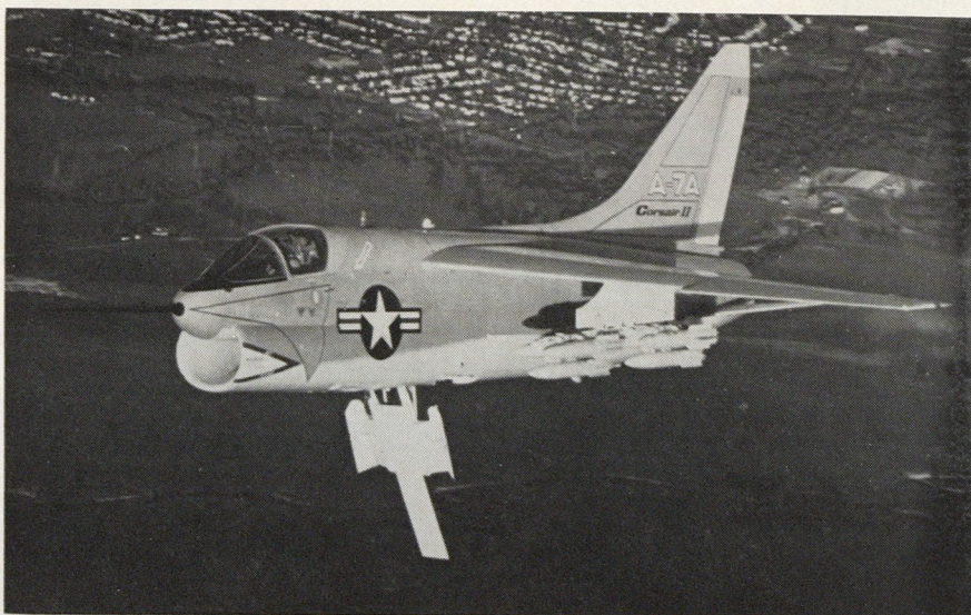
The large speed brake extended from the lower fuselage of the A-7A Corsair II is important in giving the aircraft exceptional maneuverability at low and high speeds near the ground. It allows the angle of descent to be steepened during bombing runs and improves turning performance considerably. A-7A is built by the LTV Aerospace Corp.
