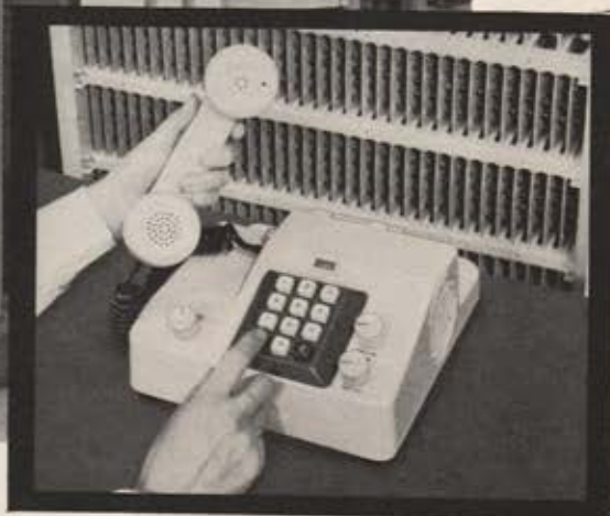
In-production solid-state Time Division Multiplex switching equipment for U.S.A.F. 412-L Air Weapons Control System. Inset: Advanced push-button tone dialing end instrument.
