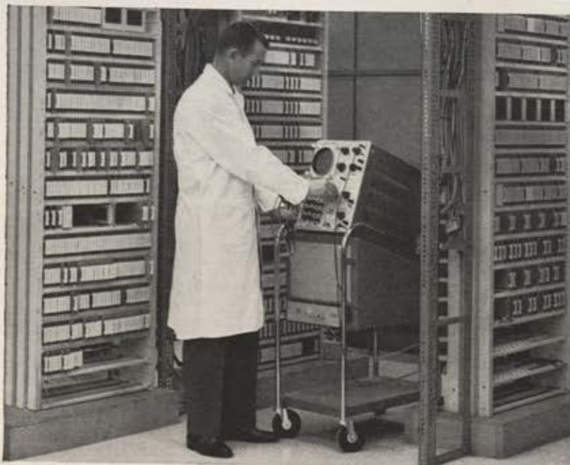
In-production solid-state Time Division Multiplex switching equipment for U.S.A.F. 412-L Air Weapons Control System. Inset: Advanced push-button tone dialing end instrument.
