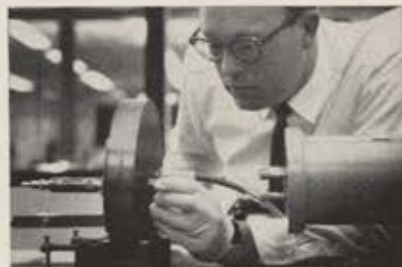
Hoffman scientist inserts KDP crystal in cavity resonator to produce electro-optical modulation of laser beam.
