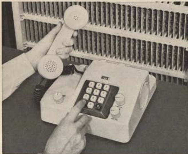
Electronic push-button tone signalling Sub-scriber Set TA-441/GTC for U.S. Air Force.
