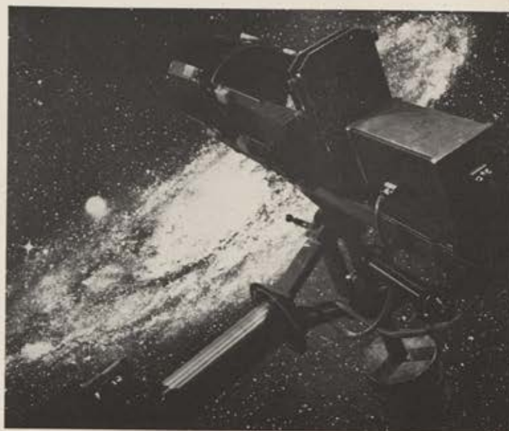
Looking to the future, Martin-designed guidance device can read star patterns, establish a pointing axis in space and thereby orient a vehicle in orbit. Instrument was designed to stress simplicity and high reliability.
