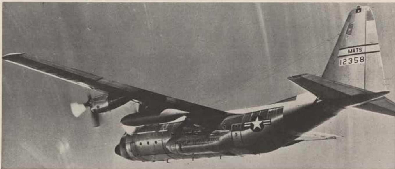
New Lockheed C-130E, with improved range and payload, flies Atlantic nonstop with normal load, Pacific in one stop.
