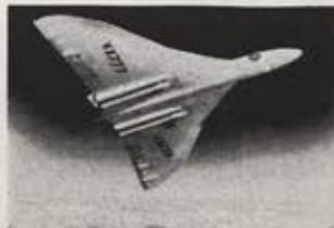
The Vulcan bomber is powered by four Bristol Siddeley Olympus turbojets.
