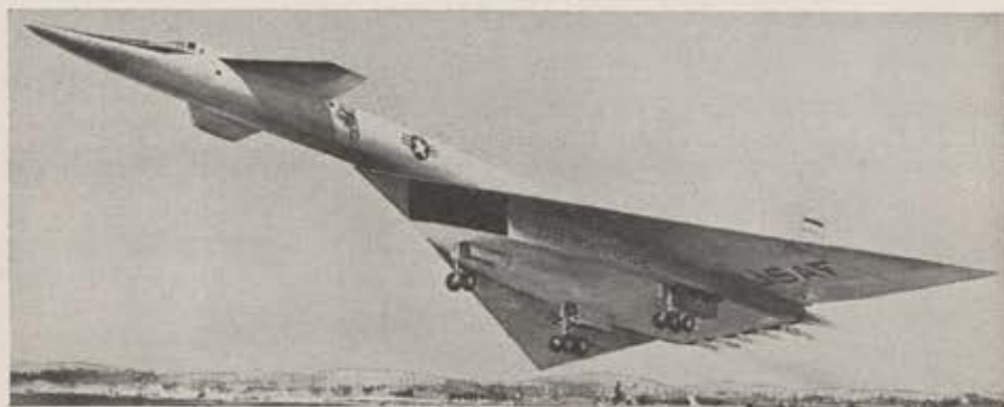
USAF's Mach 3 North American XB-70 'Valkyrie' will be powered by six YJ93 engines. A prototype aircraft is scheduled for flight tests before the end of the year.
