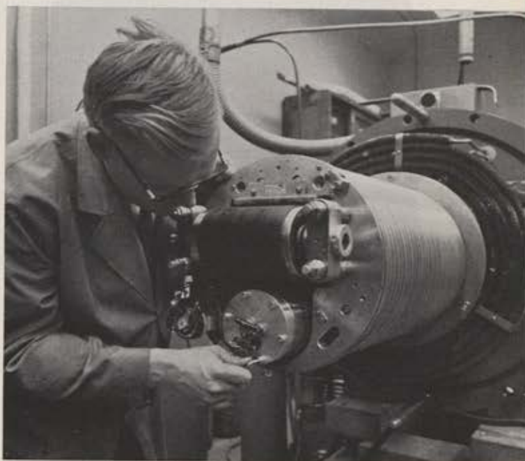
Growth and investigation of compound crystal structures is one of the major efforts of Aeronautical Research Laboratories' Solid State Physics Laboratory. Here Dr. Bernard Kulp uses the million electron volt electrostatic generator to study radiation damage effect on some crystal structures.
