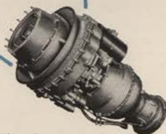
Model T72-T-2 Shaft Turbine 500 hp . . . 210 lbs.
