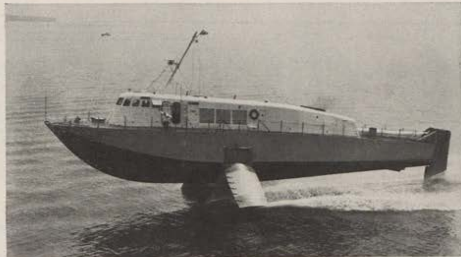
The 90-ton H.S. Denison skimmed over Long Island Sound at a top speed of 57 knots recently during her first sea trials. The developmental hydrofoil vessel was built for the U.S. Maritime Administration by Grumman Aircraft Engineering Corporation and is powered by a 14,000-shp-class General Electric LM1500 turboshaft engine. A smaller 1000-shp turboshaft, the G-E LM100, is used for low-speed harbor maneuvering when the craft is not foiborne. First commercial application is planned for 1963 when the Denison will carry tourists between Florida and the Bahamas.
