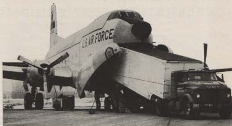
Dorsey designed and built this air-transportable trailer to house a Univac 1206 Real-Time computer and other intricate electronics equipment for missile-tracking. Remington Rand Univac Division of Sperry Corporation was prime contractor for the U. S. Air Force.
