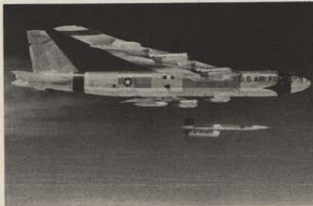
A SAC B-52 releases a Hound Dog air-to-surface guided missile, powered by a Pratt & Whitney J52 engine. With a nuclear warhead and a 500-mile range, the Hound Dog's job is to clear a penetration path for the Boeing Stratofort.
