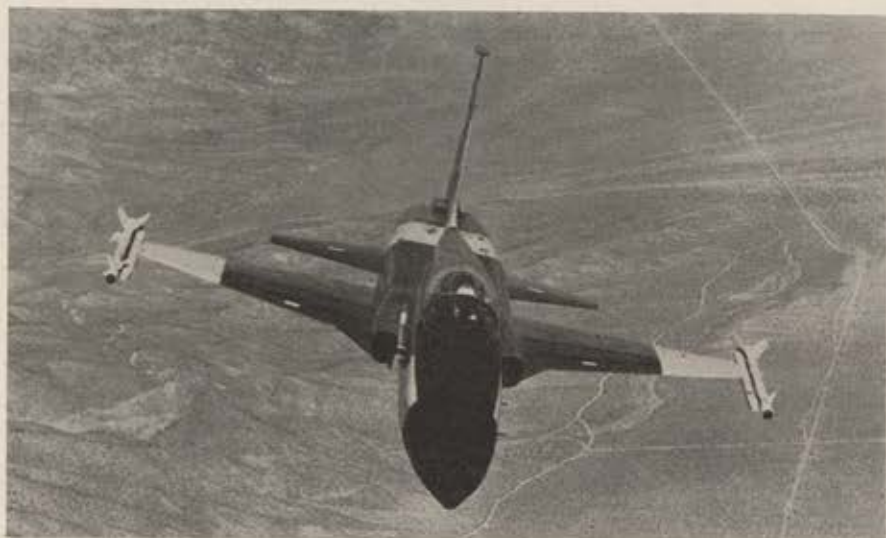
Northrop N-156, shown here in flight, will be bought by DoD for selected nations under Military Assistance Program. Powered by two GE J85-5 turbojets and able to carry 5,000 pounds externally, N-156 can fly Mach 1.4.
