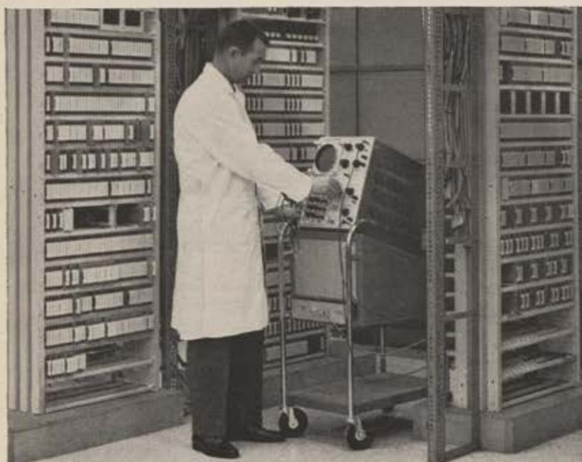
In-production solid-state Time Division Multiplex switching equipment for U.S.A.F. 412-L Air Weapons Control System. Inset: Advanced push-button tone dialing end instrument.
