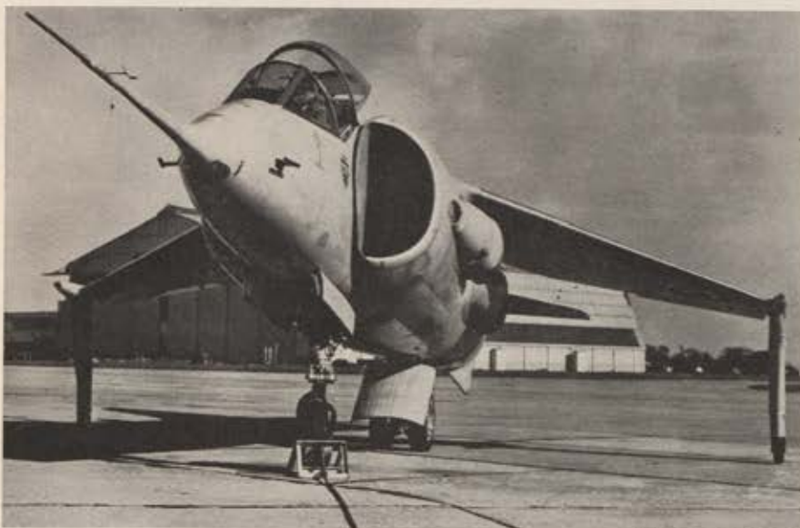
The Department of Defense is investing $35 million in the British-developed Hawker P-1127. It is a vertical-takeoff-and-landing strike/reconnaissance aircraft.
