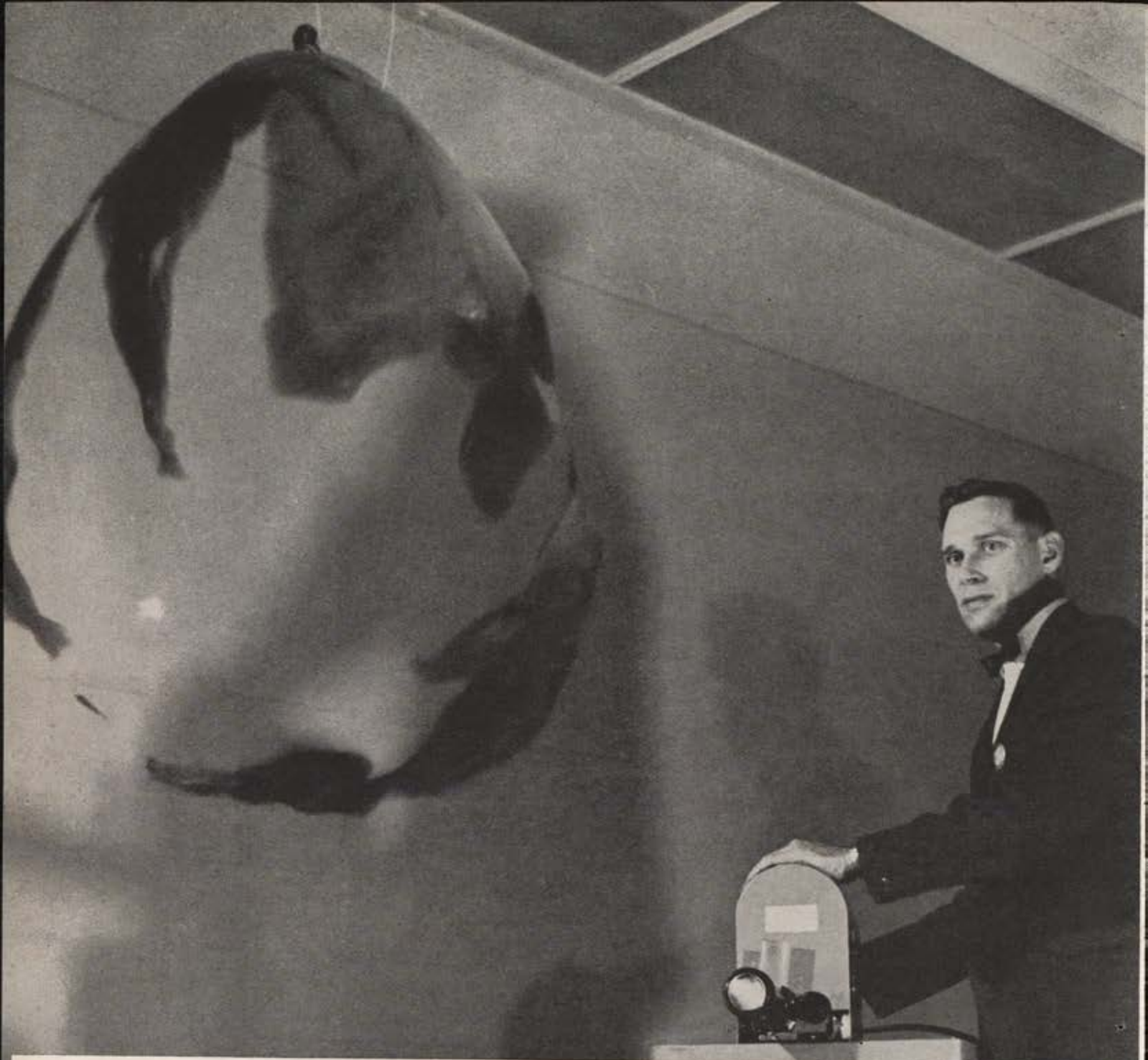
Raytheon 20 joule Laser penetrates steel to explode balloon
