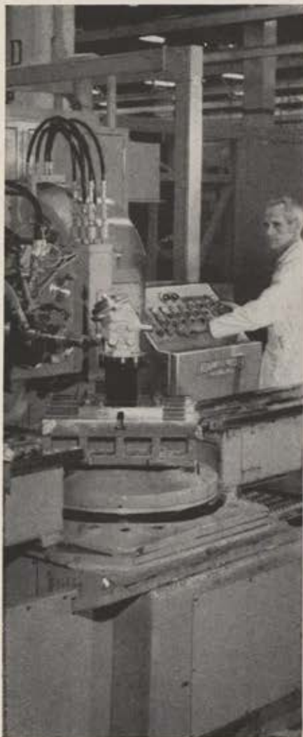
Production Machining — Volume production of precision manufacturing to space-age standards of quality and precision is achieved by use of such equipment as this numerical tape-controlled machine.
