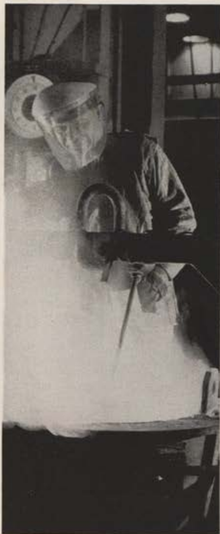
Foundry Capacity — Castings of aluminum and magnesium parts of intricate and precise design are a specialty at Wright Aeronautical. Facilities are complete for sand casting and shell molding.
