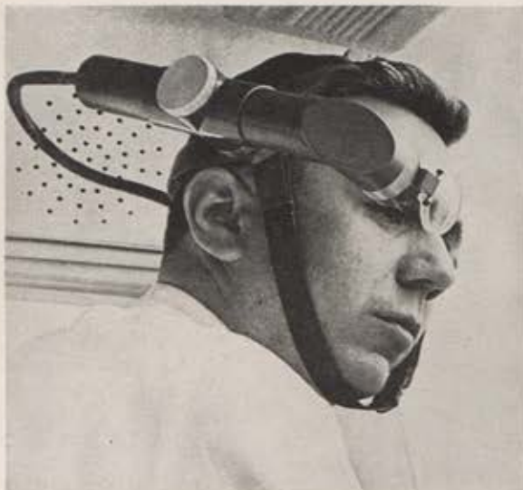
Hughes Aircraft has developed a "third eye" it calls the Electrocular . The device allows airplane pilot or other specialist to watch video image from either a remote source on the ground or a control site such as a radar screen while performing his regular duties.
