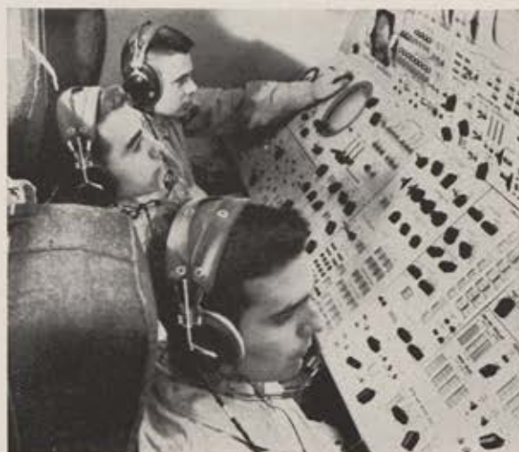
NASA spacecrew trainees will simulate round trips to the moon in Martin Company's 400-cubic-foot simulator designed for NASA's Langley Research Center, Va. Crew will "launch," make "lunar landings," and effect "earth reentry" in tests of up to a week.
