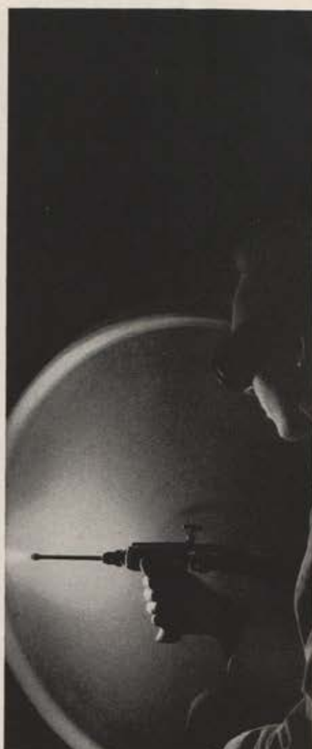
Metallurgical Research — Hot sprayings of protective ceramic coatings on experimental missile cases is one of the advanced material techniques developed by metallurgists at Wright Aeronautical.
