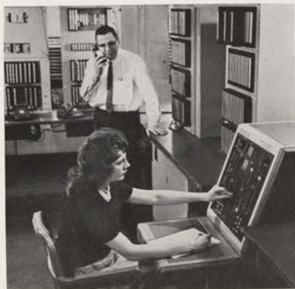
Above is an over-all view of the ESSEX (Experimental Solid State EXchange) research model set up at Bell Laboratories. Units behind the control console are only half of the total equipment.
