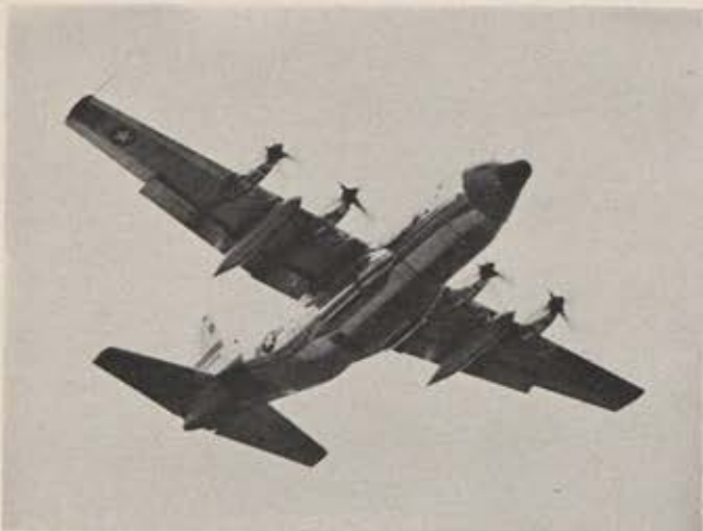
Giant ocean-spanning airlifter, Lockheed C-130E Hercules, pictured during first flight. Underwing fuel tanks will enable the plane to make nonstop transatlantic crossing carrying whopping cargo load of over seventeen tons.
