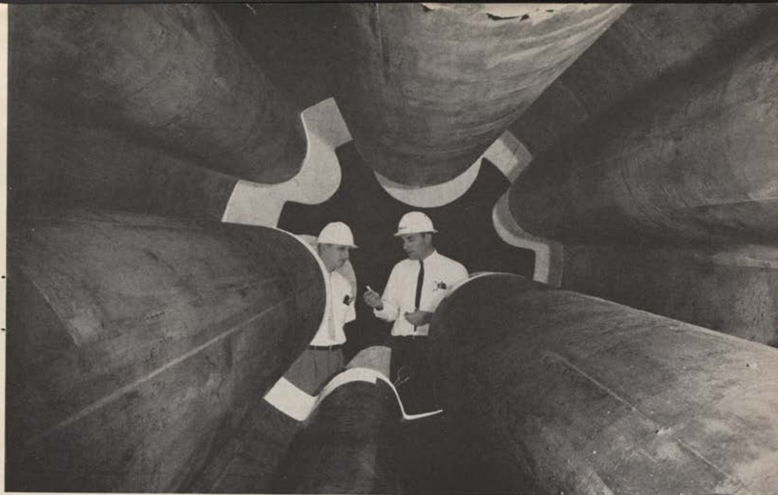
View down through the center of the world's largest solid rocket shows rubberlike propellant charge framing two Aerojet-General engineers as they stand between the center pair of the motor's segments. Rocket develops half million pounds thrust.
