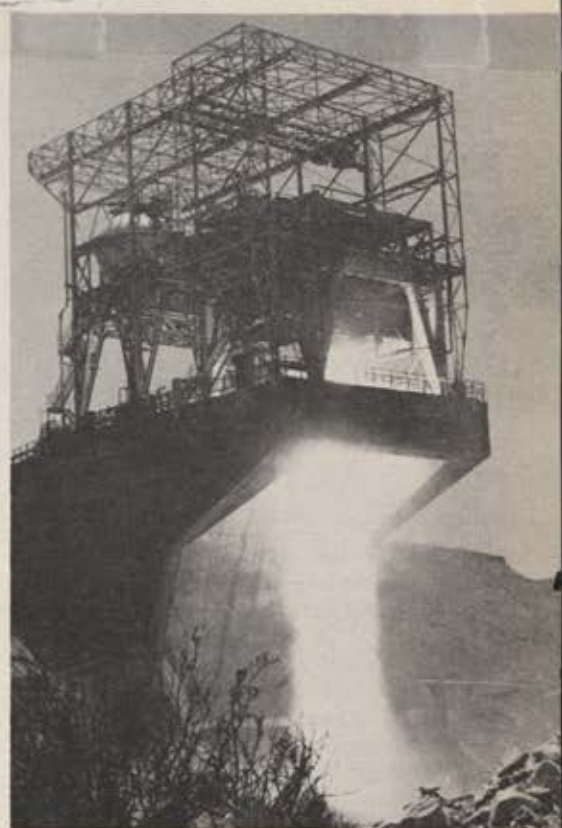
Test of F-1 1.5 million-pound-thrust rocket at Edwards AFB in California.
