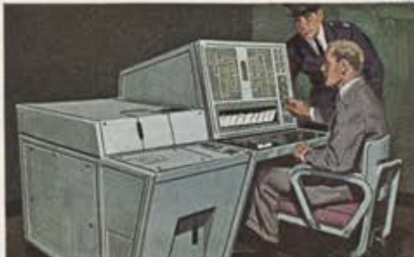
RCA's Automatic Checkout & Monitoring equipment continuously tests and checks performance of portions of the system and alerts an operator when a monitored signal exceeds certain limits.
