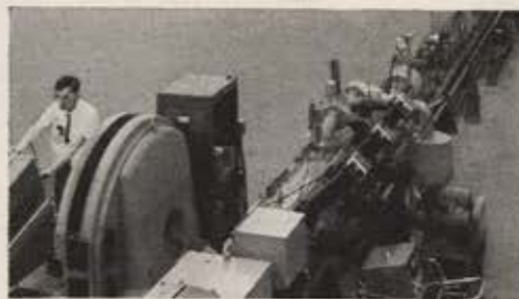
Two Light Gas Guns permit flight of hyper-velocity projectiles . . . including studies of high-speed impact, properties of ionized gases, new methods of detection and identification. If you can use facilities like these, contact DSD.
