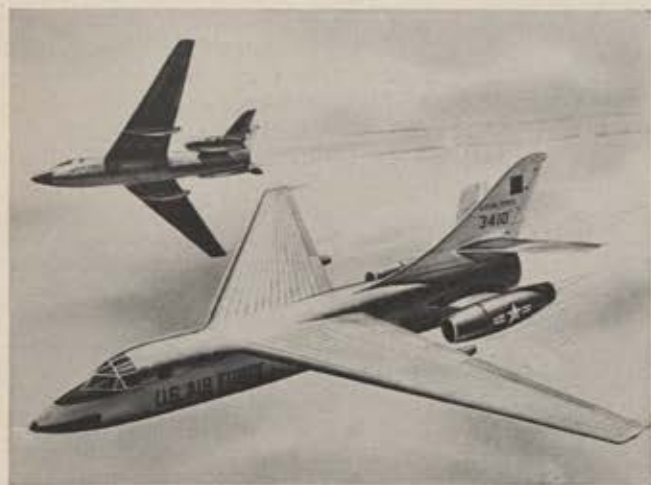
Major design details of Northrop laminar-flow control test bed are shown in artist's sketch above. The upper wing surface has spanwise slots to suck boundary layer air into the aircraft, the suction pumps are in sleeve pods under the wings, and the propulsion engines on the rear fuselage.
