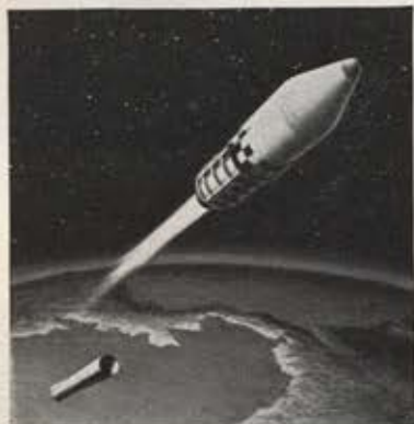
The Agena B's own engine ignites and drives it on to orbital velocity after first-stage booster burns out and drops away.
