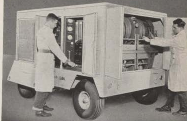
FOR AN ADVANCED FALCON MISSILE —An automatic liquid conditioner. Cools or heats electronic components, during ground checkout.
