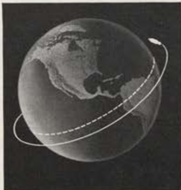
Radio signals from earth start and stop Agena B's engine to turn the original orbit into new around-the-equator orbit.
