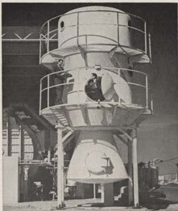
This full-scale working model of a three-man space station at Convair's San Diego, Calif., plant will be capable of duplicating space environmental conditions with exception of zero-gravity. Manned tests within model are expected to begin later this year.
