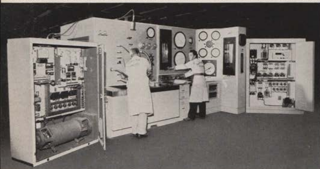
FOR THE NAVY T-56 & T-58 ENGINES —A complete jet fuel control test stand. Supplies fuel flows up to 6,500 lbs/hr at 1,500 psig. Has controllable air-flow temperature range from -65 to +300°F, accurate to \pm 1^\circ\text{F} .
