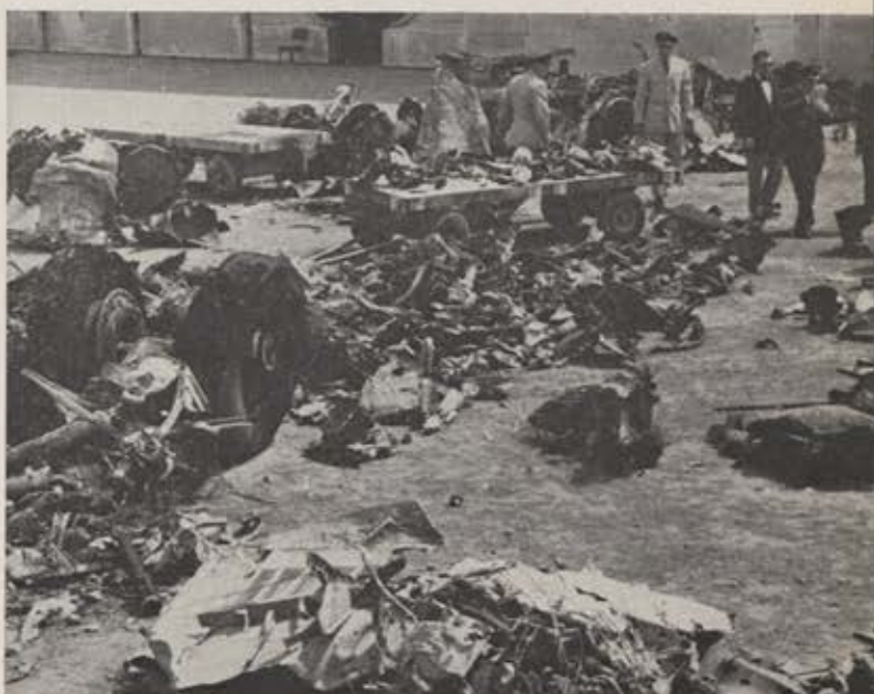
Air Force-Industry Accident Investigation Board experts study bits of wreckage collected from a B-47 which crashed at Little Rock, Ark. Although the aircraft disintegrated in midair without warning and wreckage was scattered widely, team was able to establish accident's cause.
