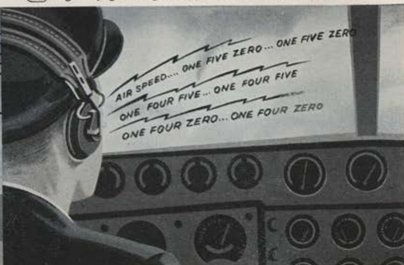
5 AUDIO CO-PILOT: An experiment in converting instrument flag warnings and selected flight data to audible signals (e.g.: calling out approach and take-off airspeeds).
