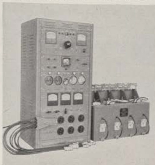
FOR THE AIR FORCE AND NAVY —A propeller synchronizer test stand for 2- and 4-engine aircraft.
