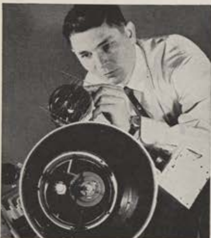
Radar for space use which uses a light beam rather than microwave radiation has been developed by Hughes Aircraft Co. The lightweight unit above is used for signaling as well as target detection.
