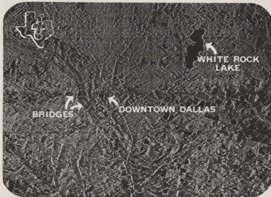
Radar image of Dallas, Texas and vicinity, taken by an all-weather, day or night combat surveillance radar system—developed by TI for the Department of Defense
