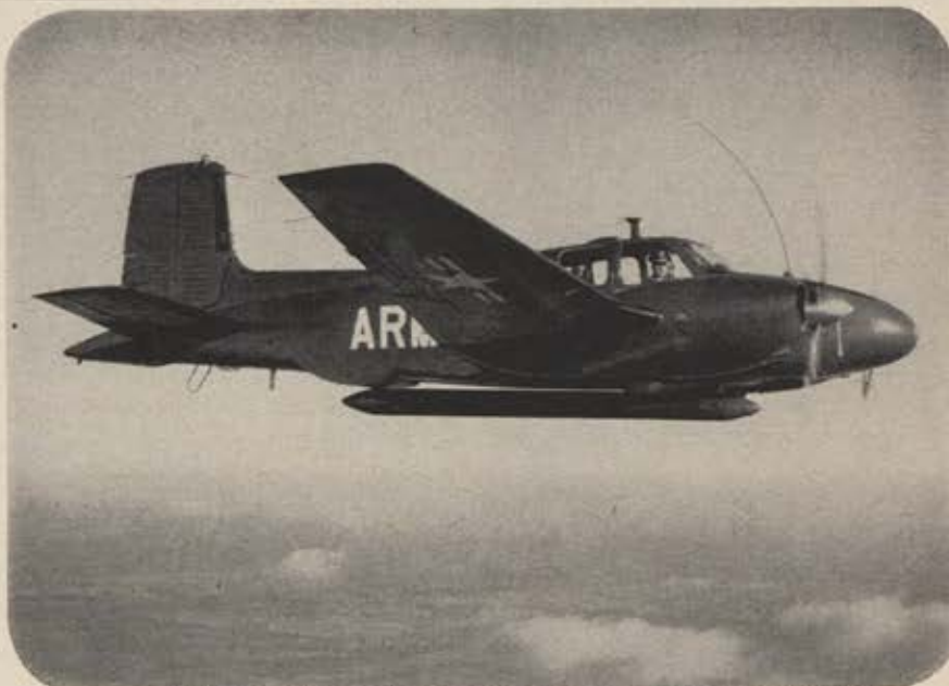
U. S. Army L23D produced by Beech Aircraft—equipped with AN/APQ-86 all-weather, high resolution reconnaissance radar, developed and built by TI in cooperation with the U. S. Army Signal Corps.
