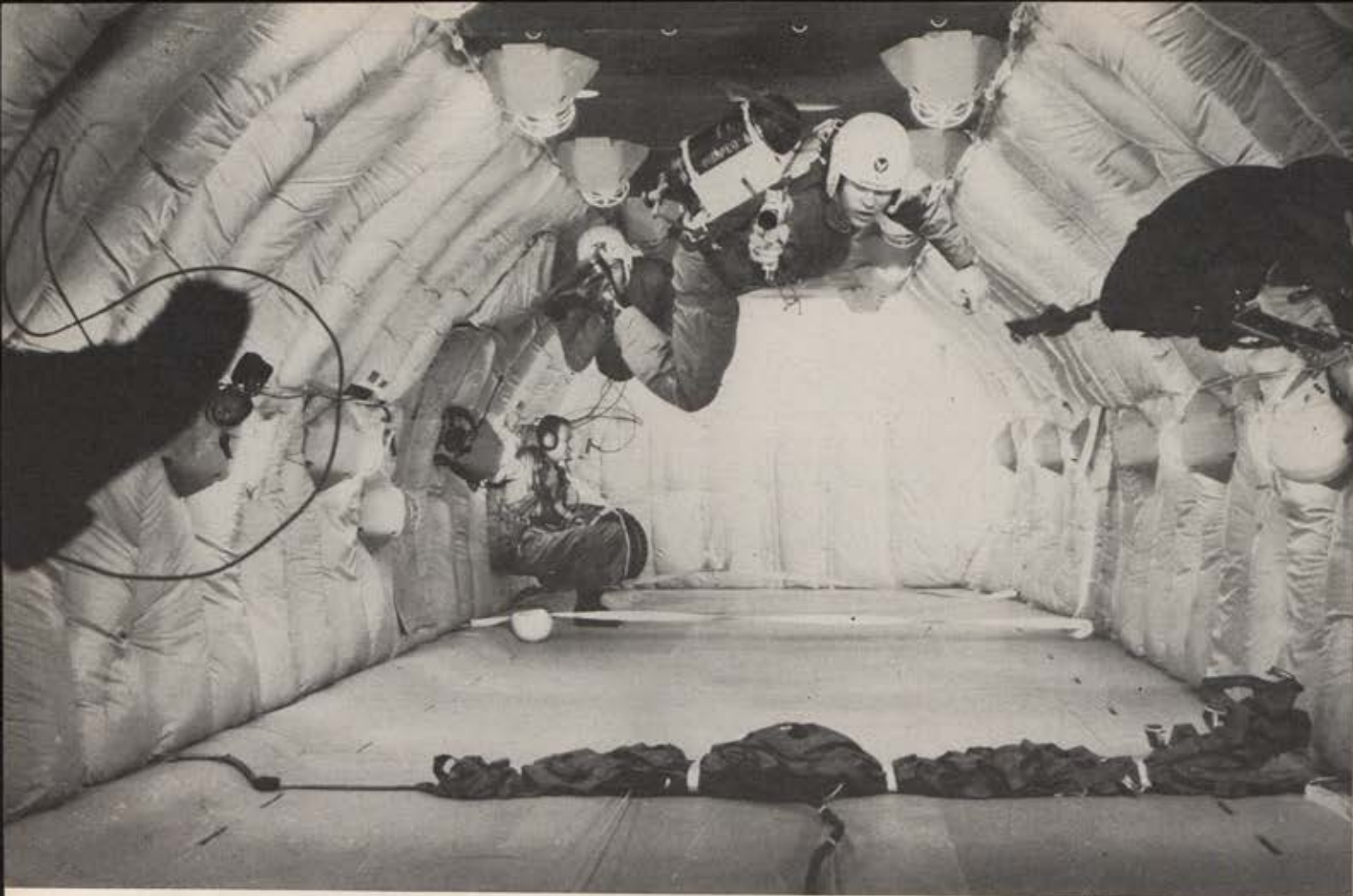
Wright Air Development Division researcher tries out a hand-held rocket to propel himself through the air during a zero-G flight aboard specially modified KC-135.
