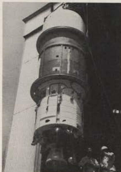
Air Force Agena-A, used in Discoverer, Midas, Samos launches, gets a checkout at Lockheed static test stand, Santa Cruz, Calif.
