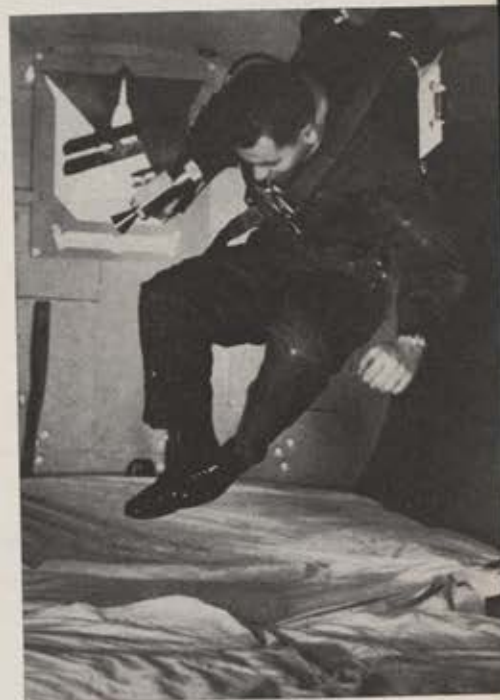
Head-down, a weightless researcher propels himself, using adaptation of an Army infantry rocket back pack.
