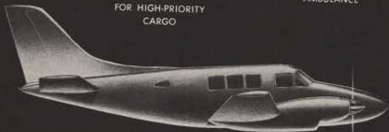
ULTIMATE PLANNED GROWTH CONFIGURATION INCLUDES TURBO-PROP ENGINES AND PRESSURIZATION.
