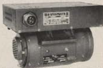
Bendix Type 32B148 Rotary Inverter delivers 115/200 volts, three-phase, 400 cps, 750 VA AC power at essentially constant voltage and frequency.
