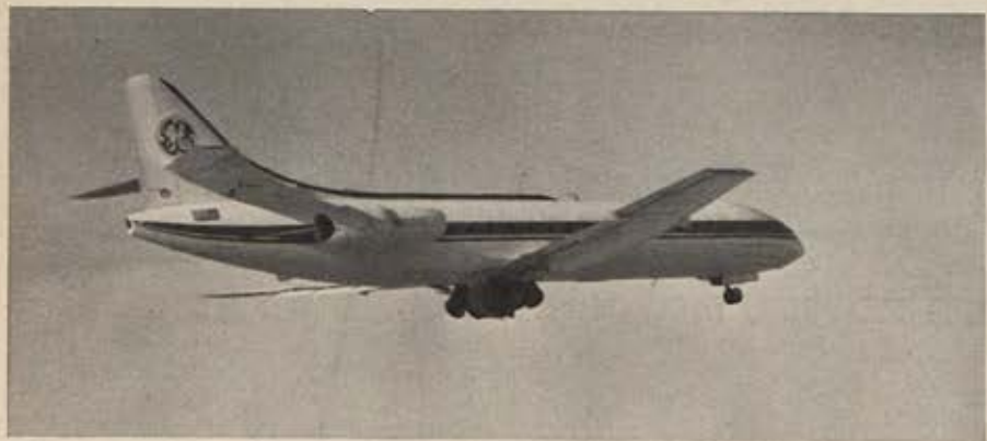
General Electric's Caravelle, equipped with CJ-805-23C aft-fan engines, completed its maiden flight Dec. 29. Production models are expected to be available in 1962.
