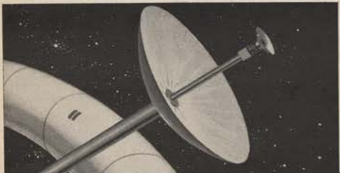
Solar concentrator with new "trumpet" condenser expands to 44½-ft. diameter. Design has been thoroughly tested for space environment.
