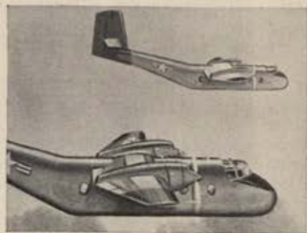
Twin T64s will power the Caribou STOL utility transport in a Navy-sponsored flight test program.
