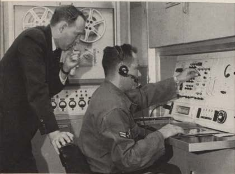
Computer work during an Atlas simulator launch with an industry expert supervising airman in training. During actual launch, electronic "brain" plays indispensable role. Here, series of mock problems are fed to airman.
