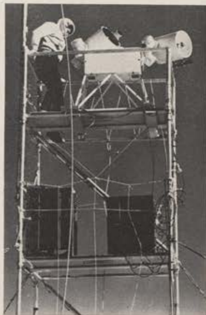
Desert tests of the experimental SOCOM, optical signaling device, show it can be used in space over distances as great as 10 million miles. System was developed for the Wright Air Development Division by Electro-Optical.
