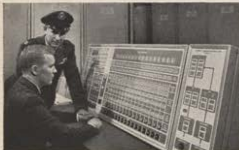
The Central Automatic Monitoring Console displays the status of the entire site, and displays equipment degradation prior to failure.
