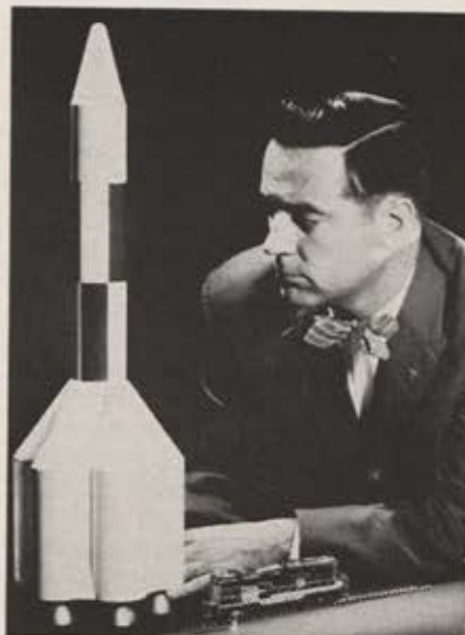
First flight tests of the NASA-Rocketdyne F-1, 1,500,000-pound-thrust, single-chamber, rocket engine are scheduled for 1963. Several types of F-1 engine clusters are being considered similar to the ones that are shown above.
