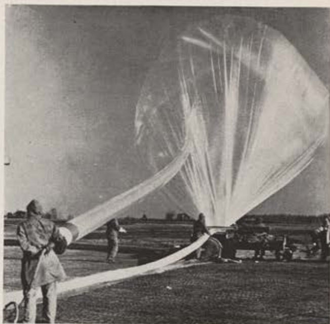
Here balloon in launch arm is being inflated prior to launch. "Bags" are made of polyethylene, are filled with helium. Balloons cost between $750 and $3,500, the helium used in one flight in the neighborhood of $500.
