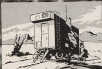
Trailer mounted refrigeration unit, 5 tons capacity
