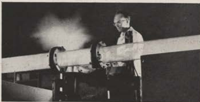
SHOCK TUBE. Industry's most powerful shock tube, designed and built by Boeing Scientific Research Laboratories scientists, creates shock waves which begin at 300 times speed of sound, then collide in tube at "slowed" rate of 80 times speed of sound. Gas temperature within the tube reaches approximately one million degrees. Studies could be important in developing effective ion and plasma-propulsion systems for use in space.
