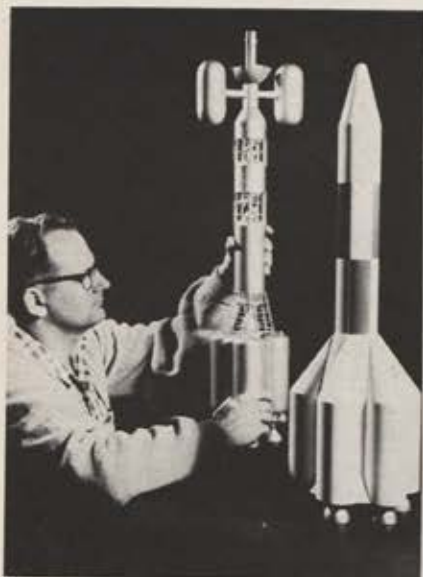
First flight tests of the NASA-Rocketdyne F-1, 1,500,000-pound-thrust, single-chamber, rocket engine are scheduled for 1963. Several types of F-1 engine clusters are being considered similar to the ones that are shown above.
