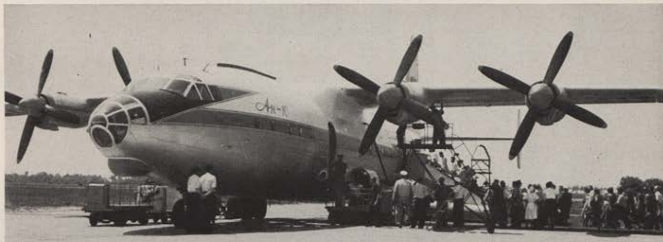
Reports from New Delhi indicate that Indians have purchased about a dozen AN-10A versions of the Red AN-10 Ukraina four-engine turboprop transport shown here. The AN-10 can take off in 2,300 feet and land on a 2,000-foot runway, but the US Air Force has a superior aircraft in this category in production. It was shown to Indian representatives in this country and met their requirements, but the manufacturer had no way of beating aggressive Red sales methods.
