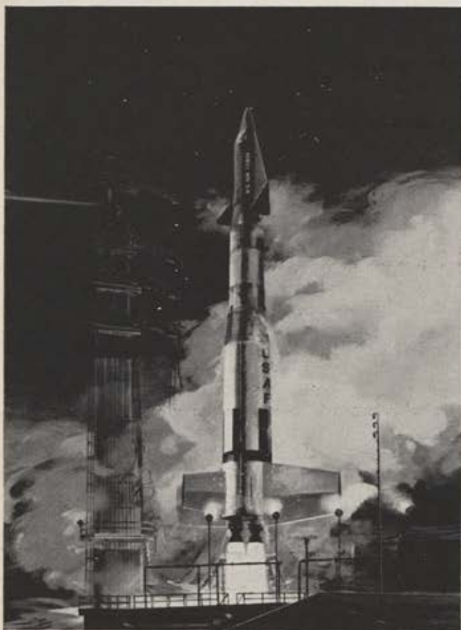
SPACE GLIDER. Artist's concept shows Dyna Soar manned space glider perched atop modified Titan ICBM for launching. In space, the glider and booster would separate, leaving Dyna Soar vehicle in piloted, near-orbital flight. Pilot could later glide to conventional landing at a selected base. Dyna Soar is being developed by the U. S. Air Force in cooperation with NASA, with Boeing as prime contractor for both the system and the glider.
