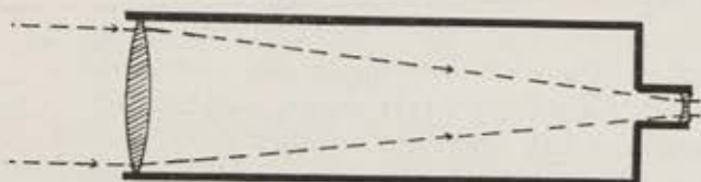
Galilean telescope, in which starlight passes in through a converging, or convex, lens. The image is viewed through a double concave eyepiece that is inside the instrument's principal focus. First Galilean telescope magnified thirty-two times.
