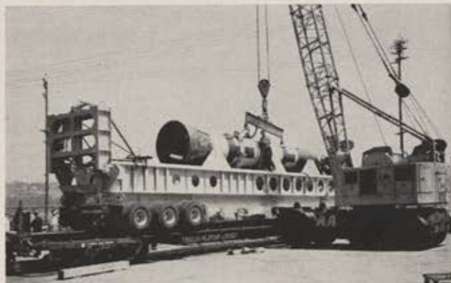
Dummy upper stages of a development test model of the Minuteman ICBM aboard railroad car at Boeing's Seattle plant.
