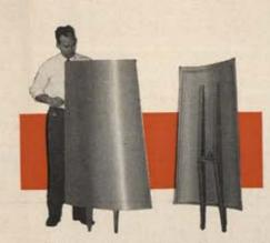
This complex speed brake for a new air weapon system illustrates Aeronca's advanced capabilities. Photo at top shows one of these units emerging from furnace after brazing cycle (indicated temp.: 2000°F.).
