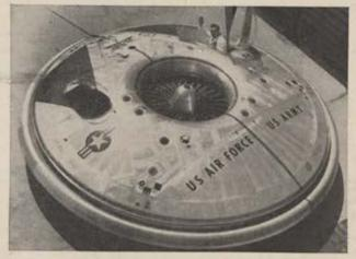
Left, a flying saucerlike aircraft called the Avrocar, a product of Avro Aircraft of Canada, which is under USAF, Army test. A VTOL craft, it is designed to hover near the ground on a cushion of air.
