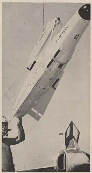
Larger than earlier Falcons, yet small considering its nuclear capability, the GAR-11 is 7 feet long, 11 inches in diameter and weighs slightly more than 200 pounds.
