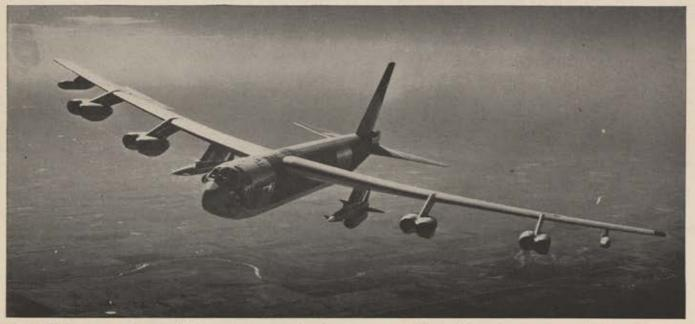
The B-52G, new version of SAC's major current bomber, can carry Hound Dog air-to-surface missiles as well as usual bomb load. The first of the new, turbofan-powered B-52Hs is scheduled for completion sometime early in 1961.
