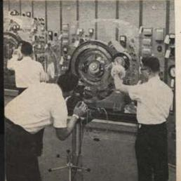
SUPERFINE TEST AND CALIBRATION. E-P checkout facilities include: Single axis and planetary sidereal test stands accurate to .005° per hour; indexing heads with an accuracy of ± 2 seconds of arc used for calibrating pendulous integrating gyros; turn-tilt stands positionable to ±5 seconds of arc; and ball disc integrator test stands accurate to .0025%. Calibration equipment was bench-mark-positioned by certified geodetic survey.
