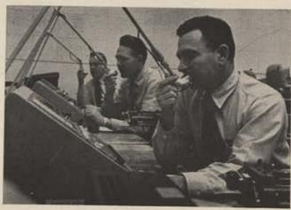
Radio operators work at control board of SAC's new singlesideband radio system known as "Short Order," System can put Hq. SAC in immediate contact with aircraft anywhere,
