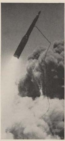
Silo-test model of Air Force Minuteman ICBM undergoes successful tethered launch from underground site, Edwards AFB, Calif., late last year. Missile capability has been prime ARDC product.
