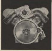
This aluminum compression ignition engine weighs only 2485 lbs. It develops 580 HP at 2200 RPM without fan or generator. No delicate field adjustments are required. It burns a variety of fuels. Liquid cooling maintains engine temperatures within optimum limits under extended high output conditions.
