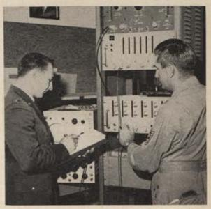
Plasmatron is used at Air Force's Special Weapons Center, Kirtland AFB, N.M., to create temperatures of up to 25,000 degrees Fahrenheit for test of materials in reentry vehicle simulations.
