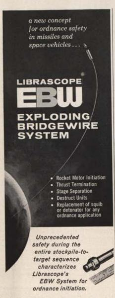
Aboard the vehicle, EBW's virtual immunity to premature initiation makes it possible to eliminate elaborate safing mechanisms. Weight of multi-stage missiles and space vehicles can thus be significantly reduced.
