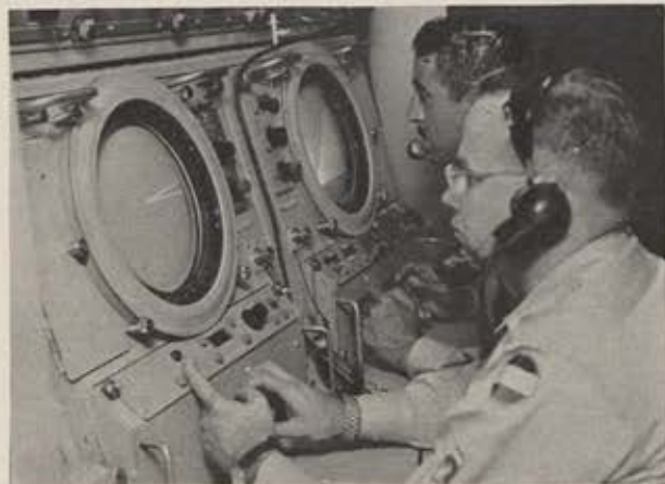
These alpha-numeric displays, developed by Hughes Fullerton engineers, can simultaneously plot hundreds of fast-moving aircraft.
