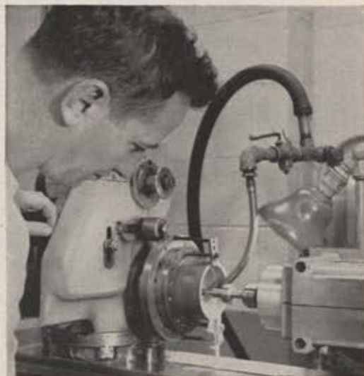
Precision ceramic envelope receives a final machining after being fired at a temperature of 1300° C. Diamond grinding and ultrasonic drilling are utilized in finishing the envelope.
