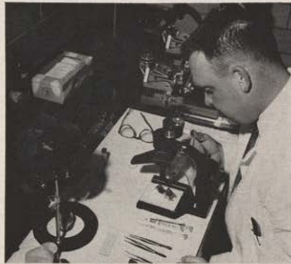
Delicacy in whisker handling is underscored by this operation in which glue is applied by hypodermic needle to enable placing whisker in holder.
