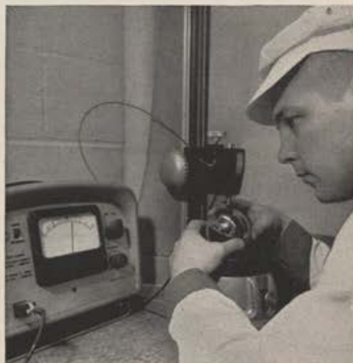
Beryllium rotor , after being machined, ground and polished, is checked for sphericity to tolerances of a few millionths of an inch!
