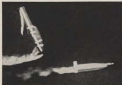
Newly released photos show Northrop Snark intercontinental-cruise missile in flight over Atlantic Missile Range. In first frame, nose cone containing dummy warhead separates from missile body. Warhead streaks toward target and the body falls away in second shot. Third view shows it in trajectory toward target. Snark, subsonic, is operational.
