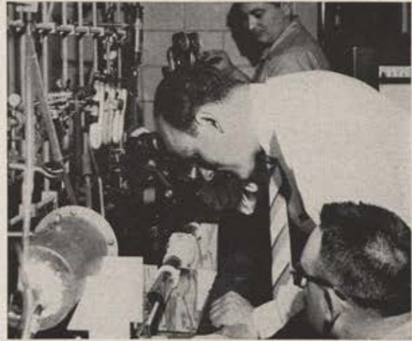
Dr. Helmut Weik watches whiskers grow, through a microscope mounted on a homemade furnace, while James J. Niles checks instrument readings.
