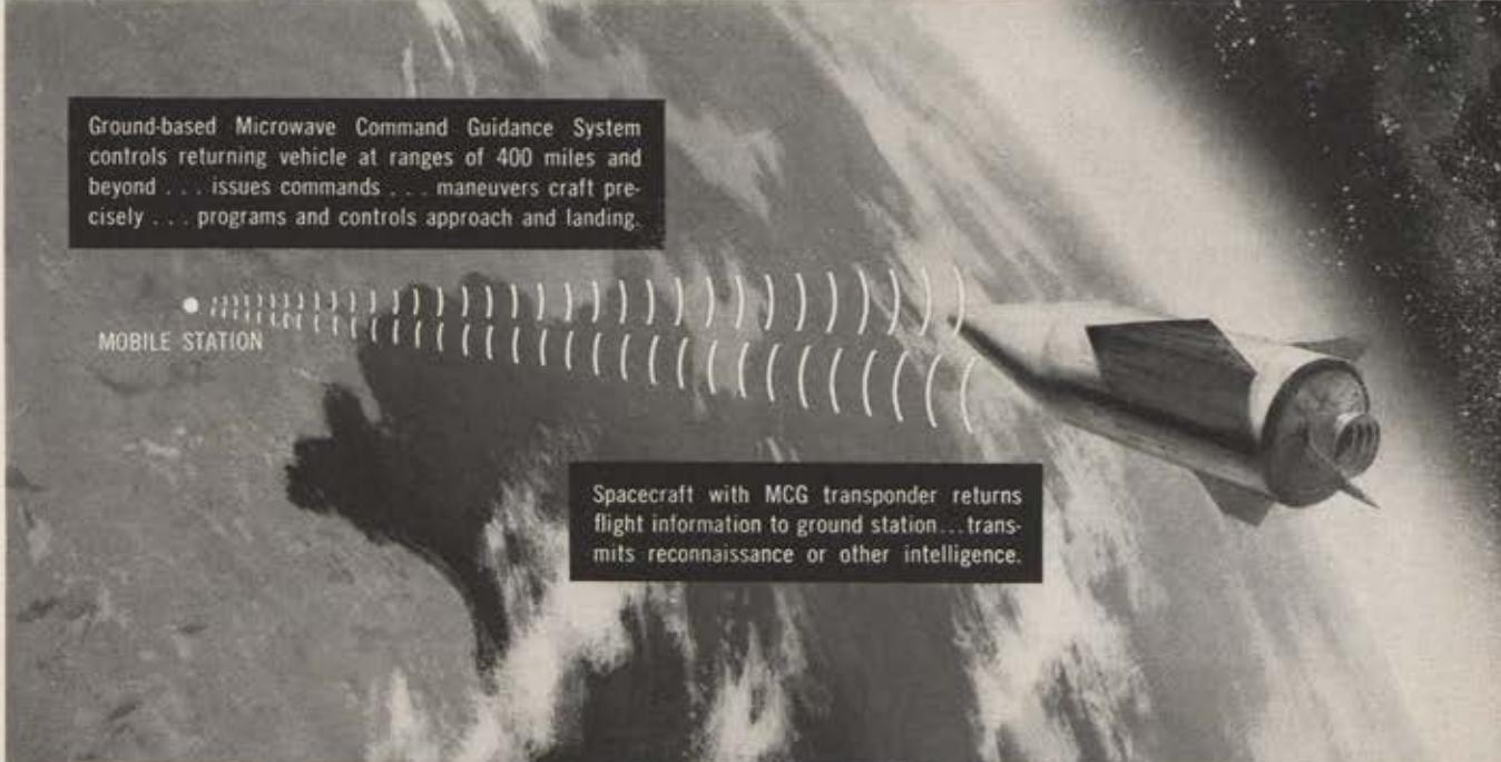
Ground-based Microwave Command Guidance System controls returning vehicle at ranges of 400 miles and beyond . . . issues commands . . . maneuvers craft precisely . . . programs and controls approach and landing.
