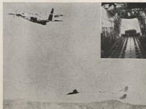
Left, a heavy-equipment drop record is set by a USAF Lockheed C-130 at El Centro, Calif., Navy base on May 12. Plane is seen here just after drop of 35,000 pounds of scrap metal under chutes. Inset is crew's view of drop from within plane.
