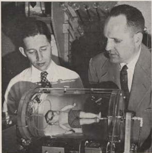
*Lockheed Human Factors Research Laboratory* specialists examine model of "null-gravity" simulator, huge revolving tank of water in which subject will be placed to gain data on human reactions to in simulation of the weightless state. At left, Dr. Raphael Levine; right, Dr. Jack Kraft.
