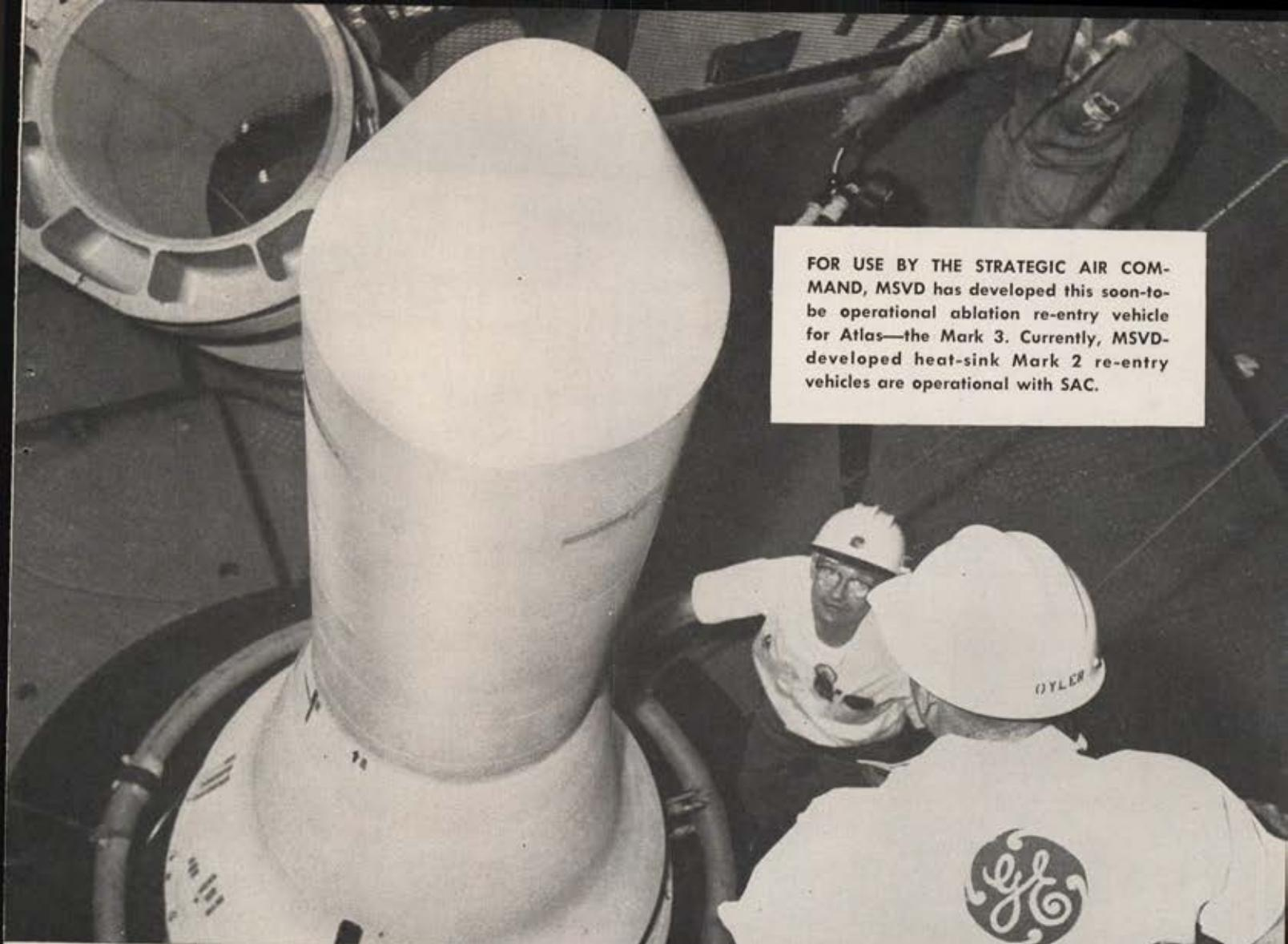
FOR USE BY THE STRATEGIC AIR COMMAND, MSVD has developed this soon-to-be operational ablation re-entry vehicle for Atlas—the Mark 3. Currently, MSVD-developed heat-sink Mark 2 re-entry vehicles are operational with SAC.
