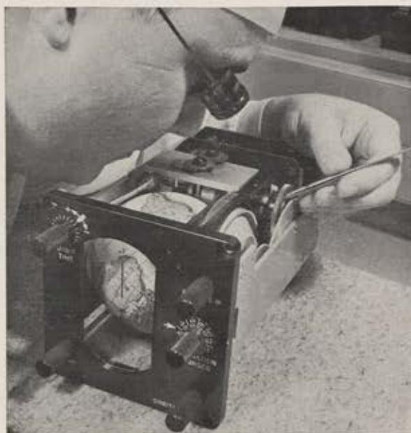
*Mercury Astronaut will watch the world turn* via this Minneapolis-Honeywell miniature globe mounted in capsule. Little globe will revolve to correspond to earth's movement, tell the Astronaut where he is, help him in the return maneuver.
