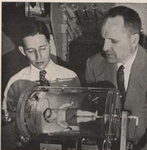
Mercury Astronaut will watch the world turn via this Minneapolis-Honeywell miniature globe mounted in capsule. Little globe will revolve to correspond to earth's movement, tell the Astronaut where he is, help him in the return maneuver.
