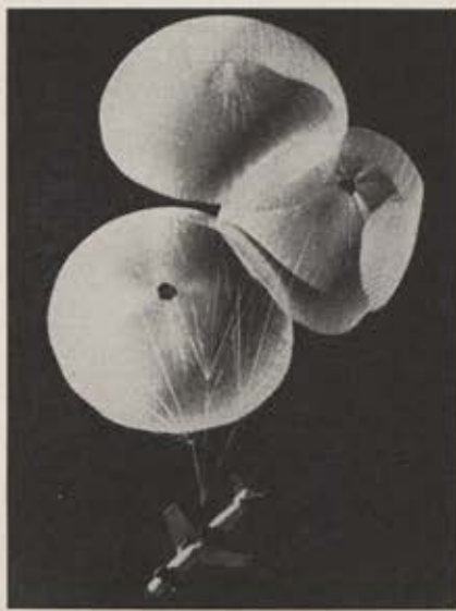
Chuting missile. Martin Mace drifts to earth beneath parachutes after flight at Holloman AFB, N. M. Missile is reused after such recoveries in Mace crew training program at base.
