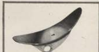
APS-94 ANTENNA SYSTEM included complete design of antenna for airborne side-looking radar.
