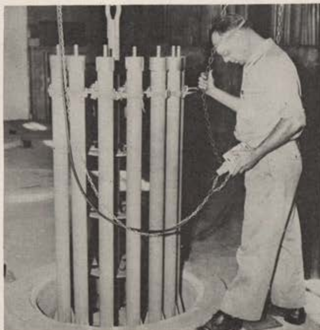
Lowering a rack of small rocket motors into curing pit at the BFG Rialto plant after propellant has been poured into the cases. B.F. Goodrich has been engaged in composite solid propellant research since 1952—in motor production since 1957.
