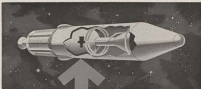
TRW's power conversion system, shown here in relative position in a typical space satellite, was developed as part of the AEC's SNAP II project under prime contract to the Atomic International Div. of North American Aviation, Inc.
