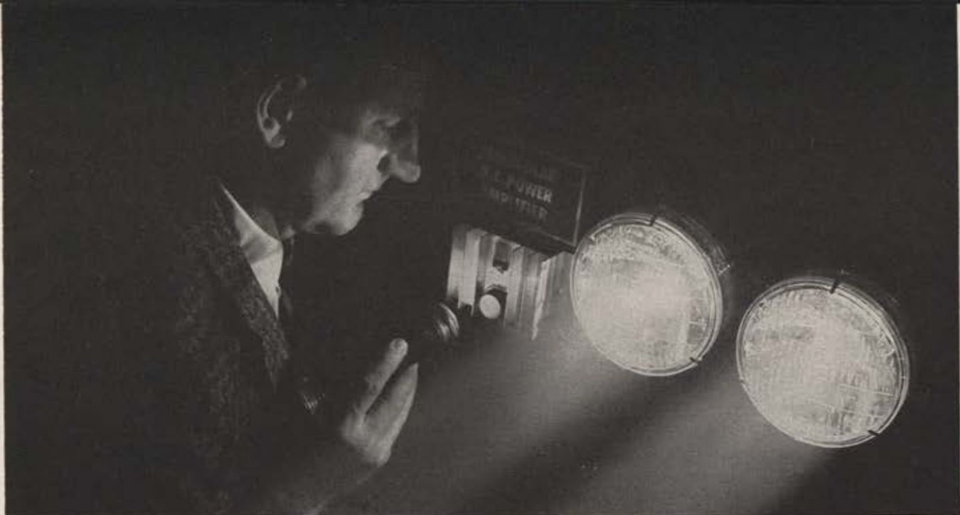
D-C AMPLIFIER: connected to a solar cell, this tiny block takes an input of 4 milliamps . . . via flashlight beam, raises it to 40-watt output.
