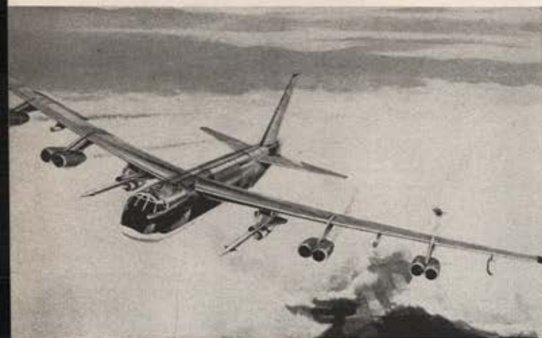
Artist's sketch, Boeing B-52H, slated for SAC in 1961. Craft is powered by eight Pratt & Whitney turbofan engines. Armed with Hound Dog, the "H" is equipped with pods containing rockets to be used as penetration aids to targets.
