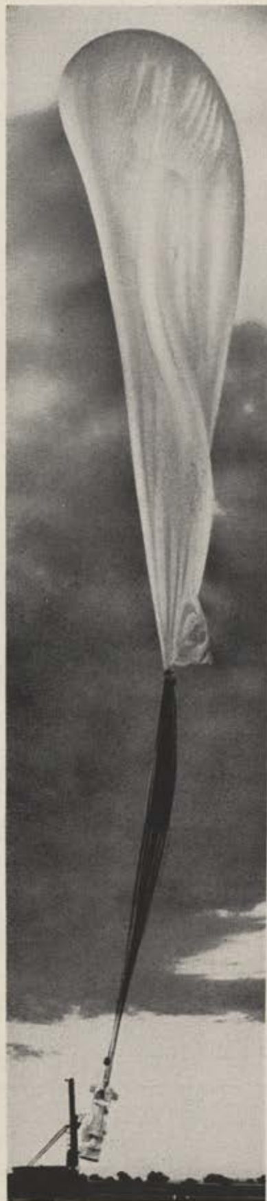
Going up for "good seeing." Unmanned balloon-observatory starts its ascent to take sunspot photos. "Project Stratoscope" is a continuing program of the Office of Naval Research and the National Science Foundation.
