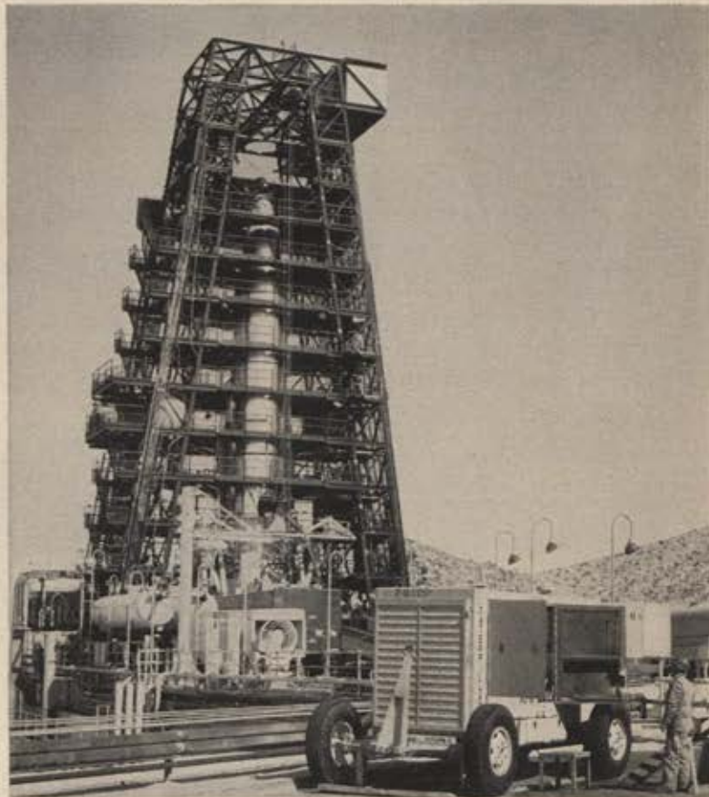
At Edwards Air Force Base in California, power for testing the precision electronic control circuits of the Atlas missile is supplied by two Cat D375 Diesel Electric Sets. They meet the triple requirement of portability, dependability and accurate control.
