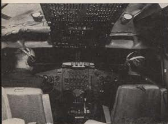
Cockpit controls in VC-137 are fewer and simpler than those in any modern four-engine piston-powered aircraft. Navigator is aft of pilot on the left side, flight engineer behind copilot.
