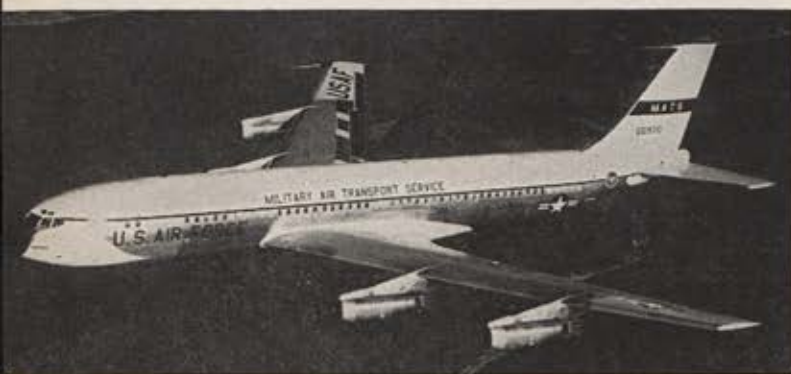
Boeing VC-137 used on Operation Monsoon is one of three operated by USAF to transport government officials. It grosses at 248,000 lbs., cruises about 550 mph at 40,000 ft.
