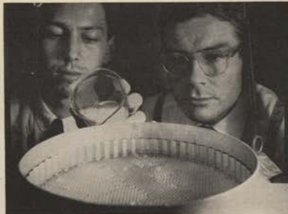
GE engineers study movement of atoms with this newly developed simulation device, which is designed to approximate behavior and interaction of particles in solid, liquid, and gaseous states.
