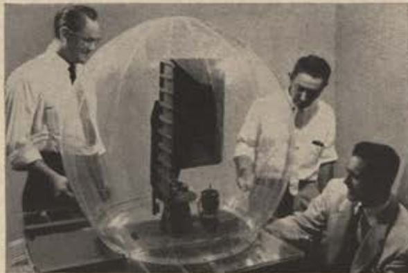
Electronic Scanning Radar system, a radically new concept in radar beam positioning, whereby range, bearing and altitude can be detected with one antenna, is currently being developed and manufactured by the Hughes Ground Systems Group.
