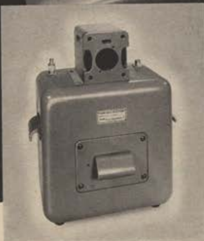
Above: Nose cone test shape traveling at 5,500 feet per second photographed with Avco Schlieren System at 0.05 \mu sec exposure. Inset: Avco Kerr Cell. Permits exposure from 0.005 to 0.1 \mu sec; available as an independent module.
