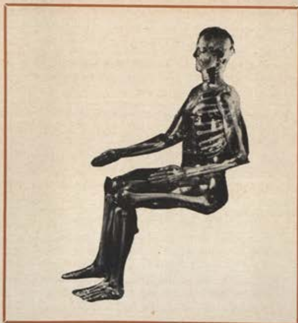
REMAB.—Radiation Equivalent Mannikin-Absorption—by Alderson Research, Inc., may precede Mercury men into space to measure radioactivity.
