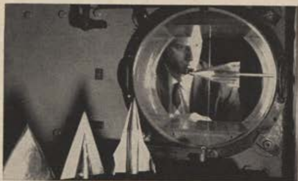
Shapes of wings to come? NASA tests models of proposed hypersonic rocket-boosted gliders.
