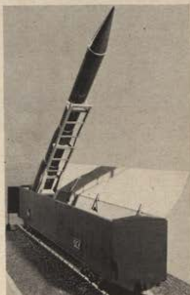
Model shows proposed railroad car launching system for missiles from railroad sidings or "stop-and-launch" sites. This model, by ACF Industries, was shown at Aerospace Panorama at Miami Beach AFA Convention.
