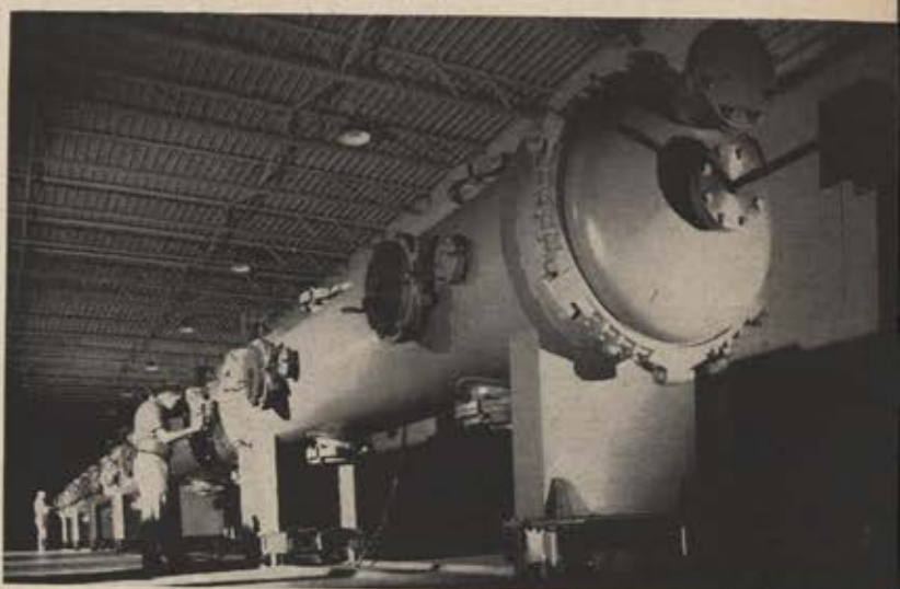
Giant shock tube blasts projectile through high-speed flight in reentry study as camera records.
