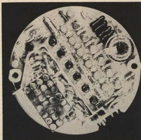
The 108-megacycle transmitter aboard Explorer VII, fired into orbit October 13 to obtain radiation data. Satellite was powered by a Juno II.
