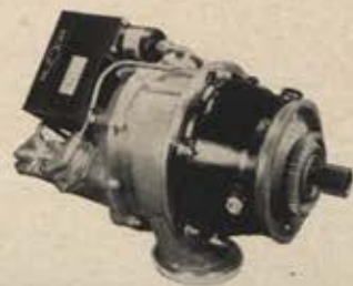
Model FAS-450-9. Weighs 44 lbs. Delivers 150 hp. Starts Thunderbirds' J-57P-21 engines (16.3 slug ft. 2 moment of inertia) in 10 seconds. Complete data available on request.
