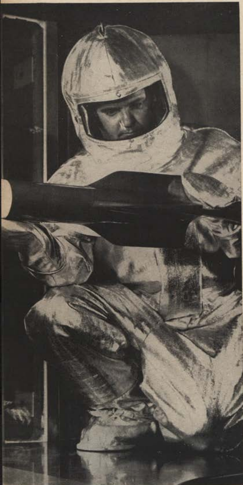
Protectively clad against 400-degree heat whipped up by 3,500-mph wind in tunnel, NASA mechanic checks rocket engine model after a test.
