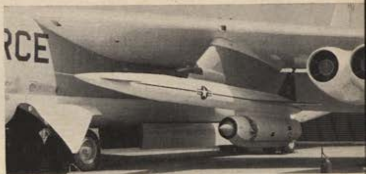
USAF's North American Hound Dog air-to-surface missile, which can fly supersonically to target after air-launch, will increase SAC B-52's striking power in years to come.
