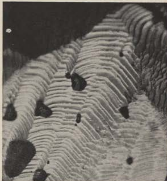
Photomicrograph of an etched silicon sphere is used in basic studies of semiconductor materials at Hughes Products, the commercial activity of Hughes Aircraft Company.
