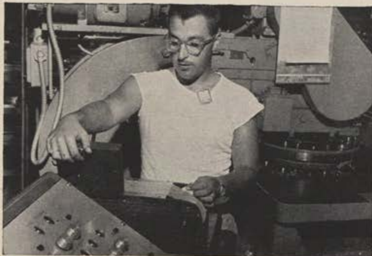
ADVANCED TECHNIQUES reduce costs and manufacturing time while maintaining high quality standards. Above, a Westinghouse-modified punch press at the Air Arm Division operates automatically by tape or dial control. It reduces lead time, cuts costs 60 to 70 percent over use of templates.
