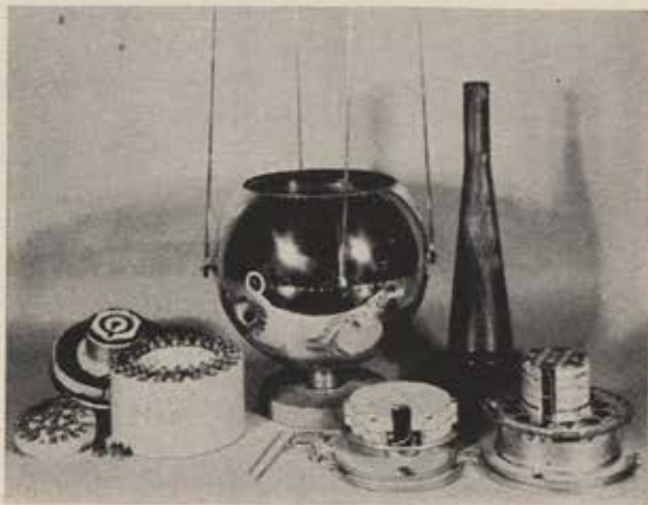
Battery packs, tubes, tracking transmitter, other innards of Vanguard III clustered around its shell.
