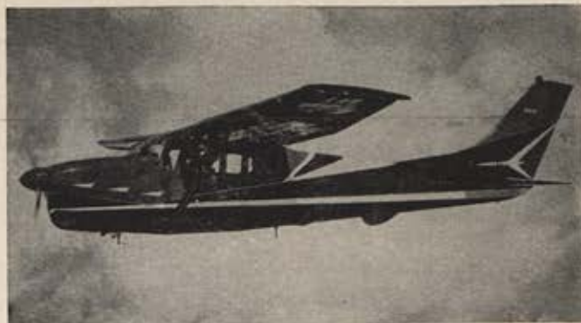
Cessna Model 210, new high-wing, retractable landing gear craft, has top speed of 199 mph, gross weight of 2,900 pounds, cruises at 190 mph at 7,000 feet. Price $22,450.
