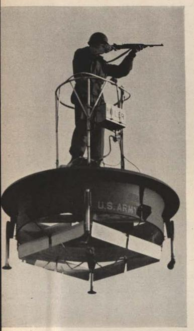
"Look, man! No hands!" Without hands on controls, pilot demonstrates hovering stability of Hiller ducted-fan "Flying Platform." Nelson H-53 engine manufacturer worked with Champion, mating plugs to engines during development stages. Now underway are three separate military ducted-fan projects—outgrawth of unconventional flight concepts proved by Flying Platform. One is development of experimental vehicle in higher speed range for Bureau of Aeronautics.
