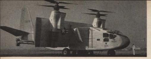
First vertical takeoff-landing transport, Air Force's 16½-ton Hiller X-18 tilt-wing, now in test at Edwards AF8. Power: Two Allison T-40 turboprops totaling 11,070 hp plus 3,400-lb. thrust Westinghouse turbojet for transition and hover control; approved with Champion Jet Igniters. (Champion pioneered jet igniter development with experimental engines in '42, remains in forefront today.) Hiller Pres. Stan Hiller predicts "inevitable conversion of entire transport system to VTOL."
