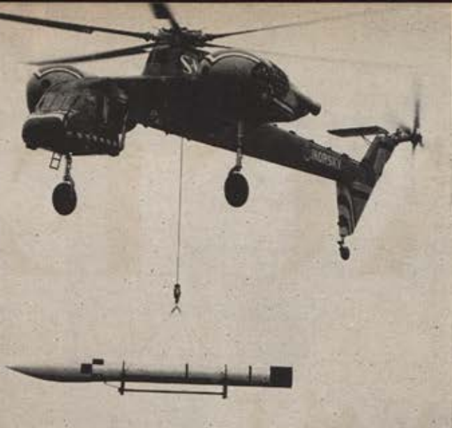
S-60 flying crane is on tour of military installations showing what it can do. Above, it hoists Army Honest John surface-to-surface rocket. Two pilots operate new S-60.
