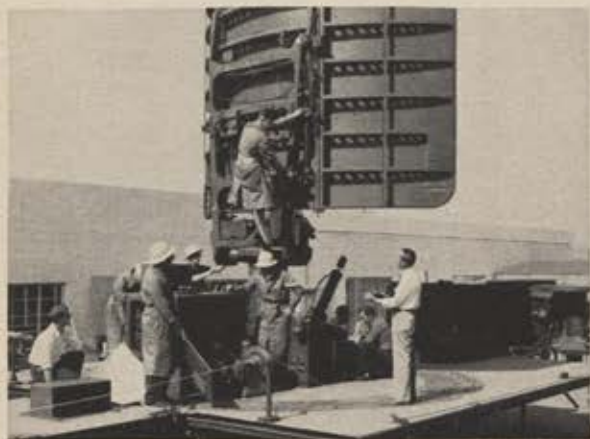
New Electronic Scanning radar antenna—Frescanar—developed by Hughes at Fullerton, positions beams in space by electronic rather than mechanical means.
