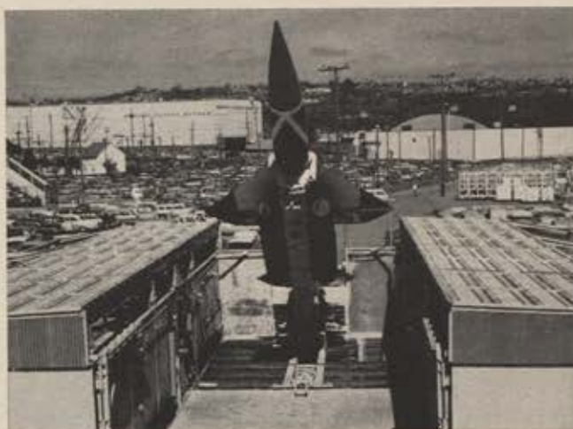
Model B Boeing IM-99 Bomarc , pilotless long-range interceptor missile currently being added to American continental defense arsenal, has a solid-propellant boost rocket and improved ramjet engines. Six-ton slabs of concrete launch shelter can be opened in three seconds.
