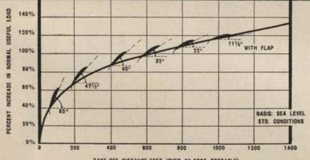
Increase in Useful Load of Tilt-Wing VTOL when operated as STOL.
