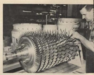
EXPERIMENTAL DEPARTMENT. This specialized factory-within-a-factory converts ideas into working prototypes. Independent engineering, tool design, progress and material control, permit self-sufficiency. Above, blades of a test cell bound compressor rotor are checked for proper balance.
