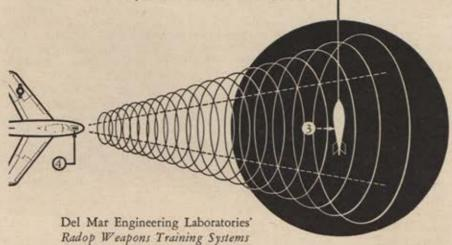
are used extensively in the training of U.S. Air Force and Air National Guard pilots. By firing rockets and missiles at inexpensive Radop Tow Targets and by using Radop Scorers to measure miss-distances in threedimensions, the Air Force saves U. S. taxpayers millions of dollars and introduces a higher degree of realism into training than is possible with other more costly systems.
