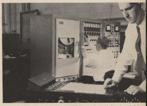
VIBRATION AND STRESS ANALYSIS data are obtained in hours instead of days with this special Westinghouse-developed Strain Gage Analyzer. From signals recorded on 14 channel magnetic tape, the analyzer plots multiple continuous curves visualizing vibration frequency and strain at varying engine speeds.
