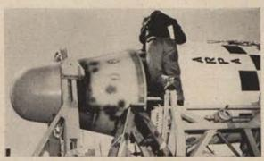
Nose of 16,000-pound Discoverer II, ARPA satellite launched from Vandenberg AFB, April 13, into a near-polar orbit, to circle the earth every 94.2 minutes.
