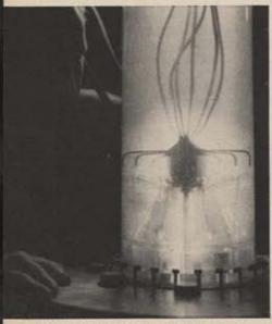
NEW FUEL INJECTOR DESIGN—fashioned from inexpensive plastic—is tested with colored water and air bubble mixture in this flow analogy test rig to predetermine its performance characteristics. Test minimizes time-consuming and costly testing previously required with expensive handmade metal prototypes.
