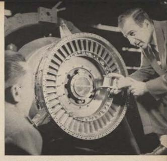
AIR-COOLED TURBINE NOZZLES permit more efficient operations at higher temperatures. Design permits air to enter through wide slots on one side, pass through interior, and leave through smaller slots along blade's trailing edge. This cools the vane and lets turbine operate at higher temperatures.
