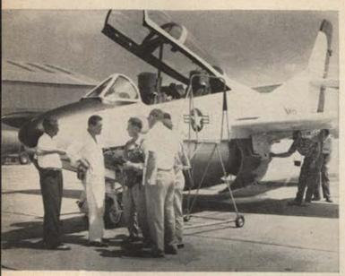
FLIGHT TEST OPERATIONS. Following thorough component testing under simulated operating conditions in the Low and High Power Laboratories, Westinghouse engineers at the AGT Division's Flight Test Center at NAS Olathe, Kansas, test all propulsion systems under actual flight conditions.
