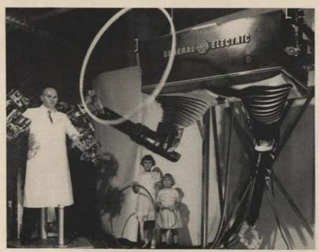
A scene from RUR? No, but almost. This is General Electric's new creature, "Handyman," developed by GE's Aircraft Nuclear Propulsion Department to handle radioactive objects, used behind seven-foot-thick concrete walls that protect the operator. Here Project Engineer Ralph Mosher manipulates Handyman in a demonstration of the robot's ability to clutch an object and simulate the action of the human hand.
