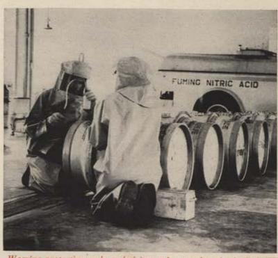
Wearing protective garb, technicians take samples of missile fuels, which are then taken to the laboratory for tests to check toxicity.
