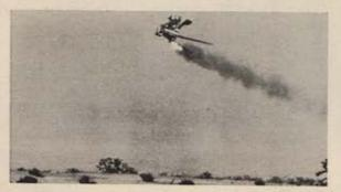
Dummy is propelled to safe height for chute home.
