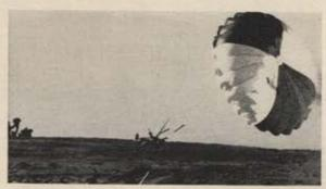
Near ground, chute opens to cushion the landing impact as the dummy ejection experiment ends.
