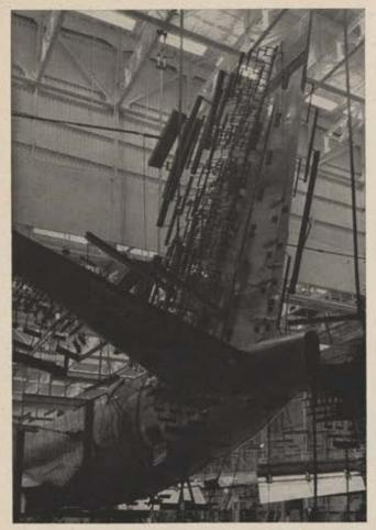
The second Convair 880 off the production line is tested for stress with a force of sixteen tons against the tail surfaces.
