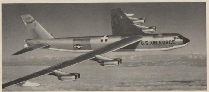
MISSILE BOMBER. Boeing B-52G, now in operation with the Strategic Air Command, is world's longest-range jet, and U.S. Air Force's most versatile long-range weapon system. B-52G carries supersonic air-to-ground missiles for in-flight launching hundreds of miles from target areas, in addition to regular nuclear bomb load. B-52G can strike several targets thousands of miles apart on a single retaliatory defense mission.
