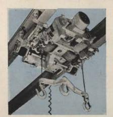
This compact, powerful fly-away hoist for the KC-135 lifts an 8,000 lb. load at 10 or 20 fpm... moves it in the plane at 20 or 40 fpm.
