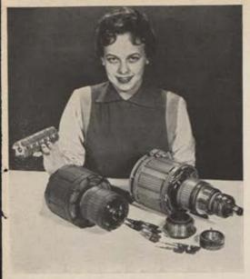
LONGER SERVICE LIFE and greater reliability result from the elimination of commutators, carbon brushes and collector rings, shown at right. A single internal rectifier bundle, held by girl, replaces them. High-temperature silicon diodes, produced by Westinghouse research in semi-conductors, make this possible.
