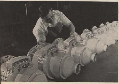
NOW IN FULL-SCALE PRODUCTION. The world's first aircraft brushless generators have a key role in advanced electrical systems provided by Westinghouse for today's military and commercial aircraft. The 40 kva units above are standard in Boeing 707 jetliners. First introduced in 1954 by Westinghouse Aircraft Equipment Dept., Lima, Ohio, these dependable generators have performed thousands of flight hours on the Boeing 707 and the Air Force B-58.
