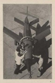
At right, XQ-2C Ryan Firebee, newest, most advanced version of jet target drones made by Ryan for the USAF soared to an altitude of 46,000 feet when launched from its B-26 "mother plane," flew twenty-six minutes, glided to earth.
