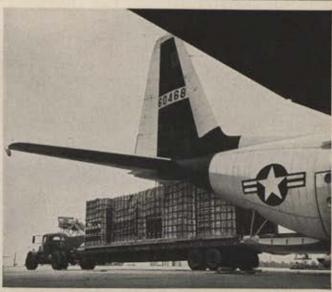
20 tons of pallet-loaded cargo can be winched in or out of the C-130 in 40 seconds. HERCULES can land, unload 20 tons, reload 20 tons, take off in 20 minutes—saving 2½ hours.
