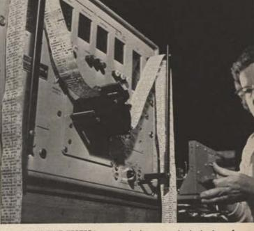
ROBOT CIRCUIT TESTER uses punched tape to check circuitry of control equipment with 100% accuracy, 60 times faster than previous techniques. Westinghouse automatic circuit-testing facilities speed production, eliminate chance of human error, improve product reliability.
