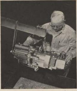
OIL-COOLED GENERATOR for Convair B-58 Hustler achieves major breakthrough of temperature barrier in electrical generator design—is cooled by MIL-L-7808 oil, having inlet temperature of 300° F. Usual generator troubles are eliminated—no brushes, commutating or slip-ring parts to wear, Results: greater economy, less frequent overhaul.
