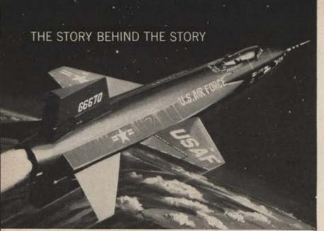
HYPERSONIC X-15, powered by a mighty rocket engine, will follow bullet-like trajectory during flight, similar to path of ballistic missile.
