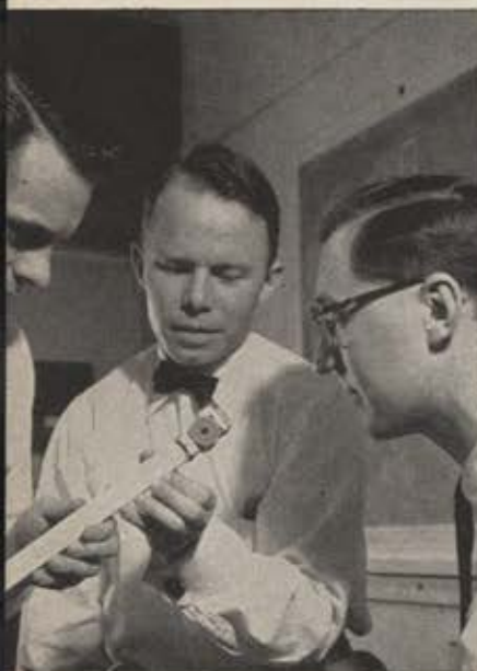
MOLECULAR SYSTEMS. A new, low-noise amplifier developed by scientists at Westinghouse Research Laboratories for Air Arm Division application. This two level solid-state maser is one aspect of a broad Westinghouse program of molecular engineering for radar and other electronic systems of the future.
