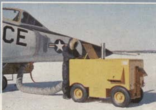
HERMAN NELSON portable heating and ventilating unit for the F-102. Each system presented a different problem; each required specially designed equipment. For each, Convair turned to AAF Defense Products Division.
