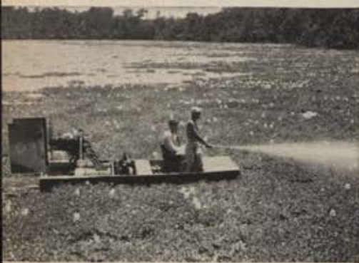
Airboat eradicates waterway-clogging hyacinths with spray-hose.
