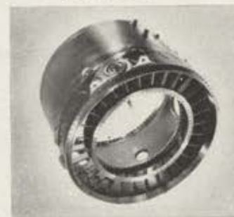
Jet engine case assembly
