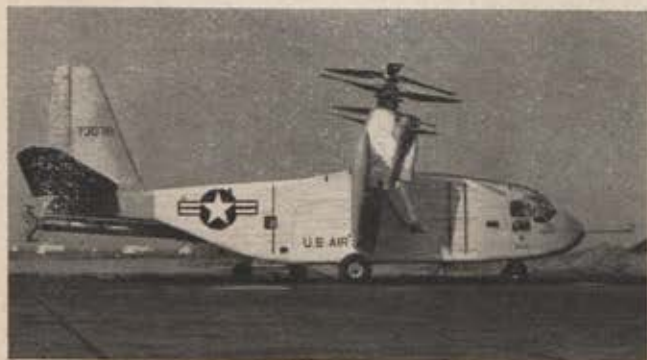
The X-18, Hiller tilt-wing research transport, rolls out, with its wings in the ninety-degree position, for VTOL.
