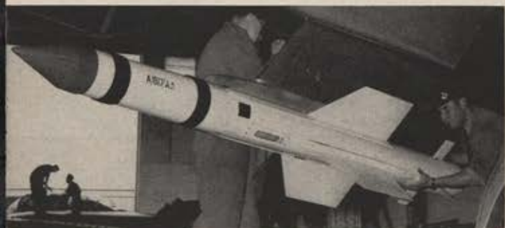
Left, de Havilland Firestreak, infrared homing missile, is loaded on a Gloster Javelin all-weather fighter. Plastic covers missile's eight-panel glass nose. Right, two of the heat-seekers aboard an English Electric Lightning interceptor.
