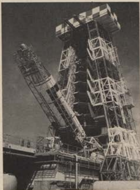
3. Slowly, carefully, Atlas is raised into position for firing. Specially built cables are used to do this delicate mission.
