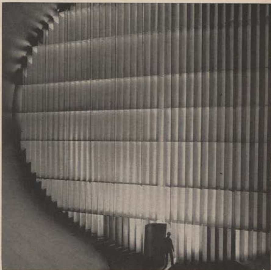
AEDC technician at bottom of photo is dwarfed by the fifty-five-foot diameter of the Propulsion Wind Tunnel. Giant vanes help decrease turbulence as the air-flow is turned ninety degrees inside the transonic circuit of this huge tunnel.
