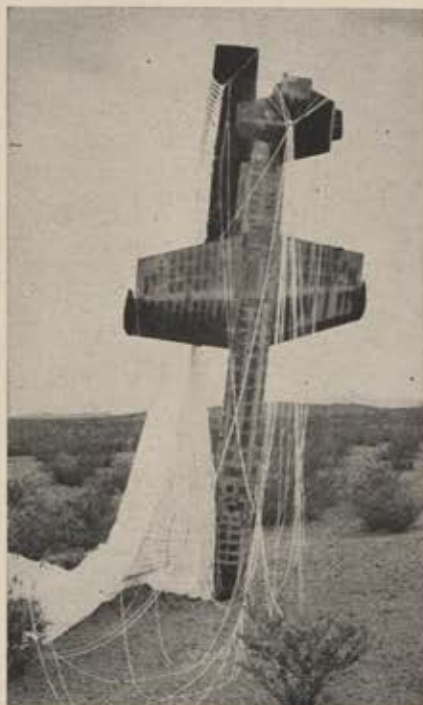
Bright yellow paint job on Lockheed's X-7 was burned black by searing air friction heat during high-speed test.
