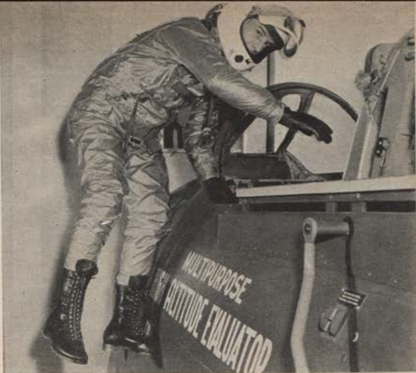
To test reliability of protective equipment, Dr. Edwin G. Vail, WADC, project scientist, enters an F-36 cockpit in the altitude chamber. He is wearing the XMC-2 full-pressure suit, to test ability to provide him a liveable atmosphere.
