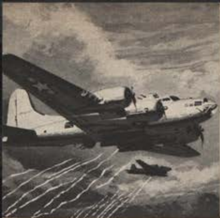
1942 First effective radar countermeasure was "Window," code name for thin strips of metal foil which reflected spurious radar echoes when dropped from Allied bombers, confusing enemy radar operator.
