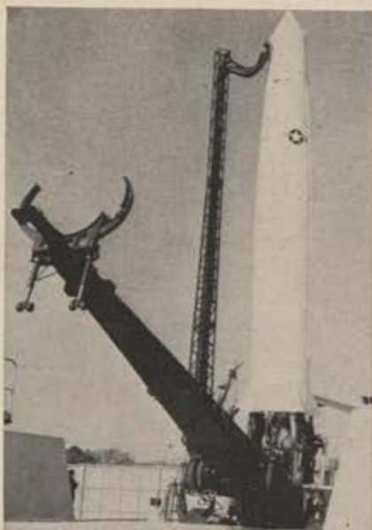
Transporter, built by Food Machinery & Chemical Corp., erects Thor IRBM to firing position at launching site.
