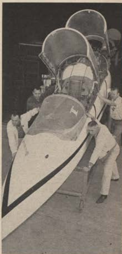
New Northrop T-38 prototype fuselage section being rolled out after rigid instrument check prior to its high-speed rocket-sled testing at Edwards AFB. It will be flight-tested late this year.
