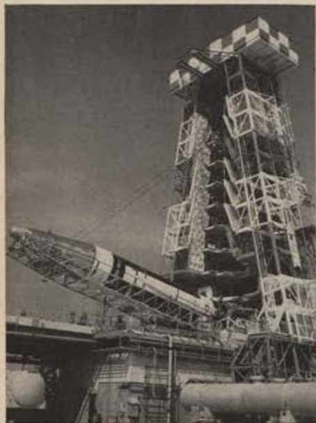
2. Atlas carrying trailer backs up to launching platform at Cape Canaveral and the "bird" is mated to waiting tower.
