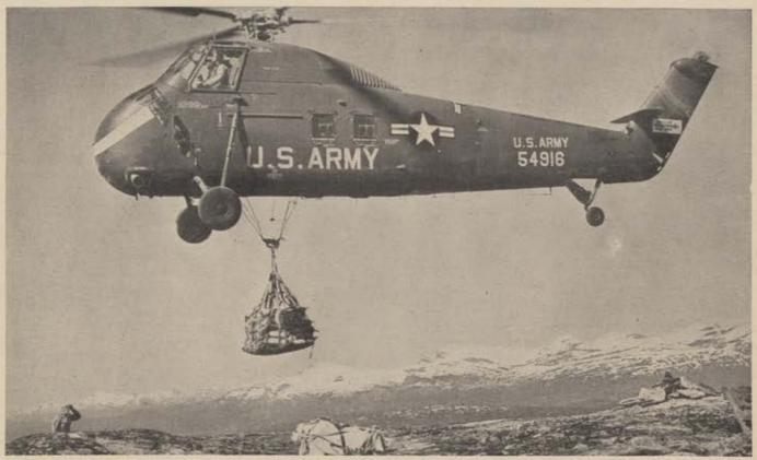
45 TONS PER HOUR—In northern Norway, pilots of the U. S. Army's 8th Helicopter Battalion carried loads of building materials, steel, electronic equipment, and even dynamite to mountain-top sites of micro-wave relay stations. The H-34As (Sikorsky S-58s) delivered their cargo at the rate of 1½ tons every 2 minutes.
