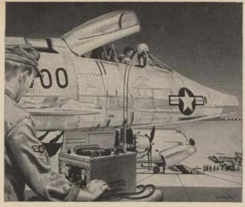
TEST INSTRUMENTS Bulova's rugged Tachometer Tester for all jet and reciprocating systems meets MIL-T-945A requirements—is accurate to 0.1% with engines on or off. Simple to operate and maintain, this field unit also serves in maintenance depots. Precise Bulova testers include the dual purpose Torqmeter—a dynamometer or calibrated torque source
