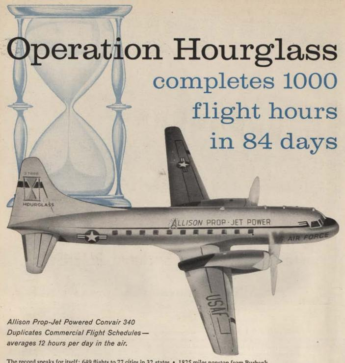
The record speaks for itself: 649 flights to 77 cities in 32 states • 1825 miles nonstop from Burbank to Indianapolis in 5 hours, 40 minutes • 12 hours flight-time each day—for 84 days—with only line maintenance on engines and propellers • Routine cruise—360 mph at 20,000 feet • Specific fuel consumption well within specification from sea level through 20,000 feet • Oil consumption—10 gallons per engine in 1000 hours.
