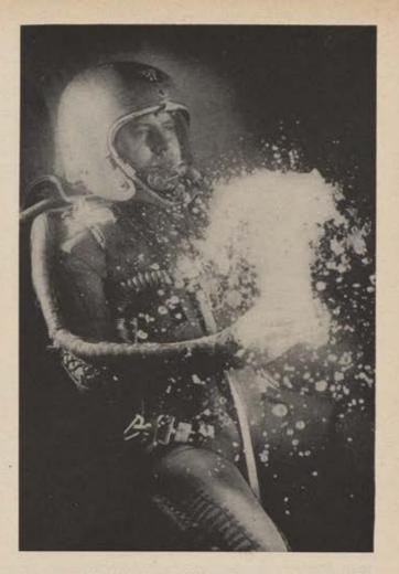
At super-high altitudes, explosive decompression would be fatal to unprotected airmen. Drastic reduction of atmospheric pressure releases gases in liquids, causing "boiling" as illustrated here in simulated high-altitude chamber, with beaker of exploding fluid held by experimenter.
