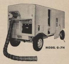
MODEL G-7 Ground Support Air Conditioner. Made for Convair Div., General Dynamics Corp. for use with Atlas Missile. Self sustained, air cooled, electric motor driven. For cooling, heating, dehumidifying, filtering and ventilating air. Capacity-360,000 B.T.U/hr. cooling; 245,900 B.T.U/hr. heating. Automatic airflow from 60 to 120 lbs./min. Automatic temperature control from 40° to 60°F. 0 to 24" water column gauge pressure.
