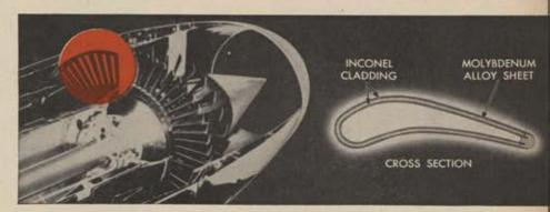
The first stage turbine nozzle vanes (outlined in red) were chosen for initial testing as they are subjected to the highest temperatures and are most susceptible to thermal shock.
