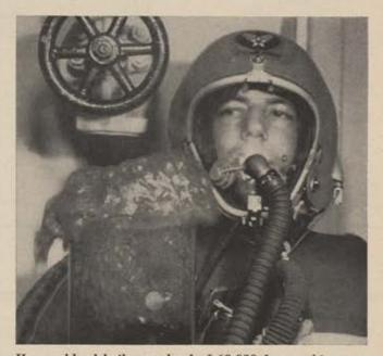
Human blood boils at a level of 63,000 feet, making protective pressurized clothing mandatory. Pictured is an experimental demonstration—using simulated human blood—of this space-travel hazard. This experiment was carried out by personnel at the School of Aviation Medicine.
