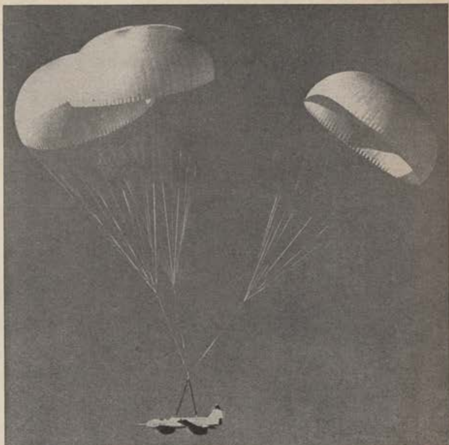
Until recently, the USAF Martin TM-76 Matador jet-powered guided missile had been a one-shot weapon, plunging to destruction at the end of its flight, but with a new kit developed by Martin, the Matador can now be recovered after use by means of controlled drag chutes, operated by an MSQ radar command system. The new system is a boon to post-flight examination, will aid training.
