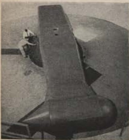
Huge centrifuge to be used at Convair's Astronautics Division for testing of ICBM components was made by Rucker.
