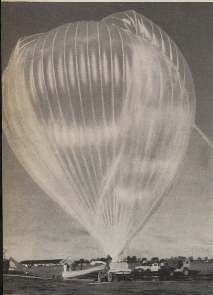
This Project Farside polyethylene balloon is identical to the one used in the actual rocket flights. Here it is being readied for a test ascent. Its load is an exact replica (size and weight) of the platform and rockets which were carried to 100,000 feet at Eniwetok Atoll.
