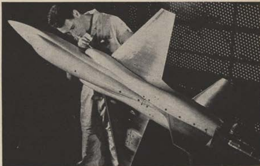
Test model of Northrop's T-38 supersonic basic trainer is shown preparatory to testing in the 1,000-mph wind tunnel at the Cornell Aeronautical Laboratory.
