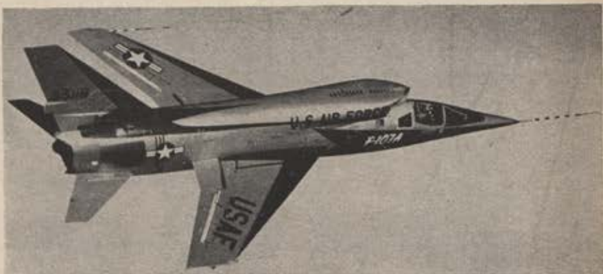
North American's F-107A single-engine jet fighter-bomber can exceed Mach 1 in a vertical climb. Spoilers on upper and lower wing surfaces rather than ailerons are used for lateral control. Overhead inlets above canopy admit air for the Pratt & Whitney J-75 engine. NACA is flight-testing the fighter at Edwards AFB, Calif.
