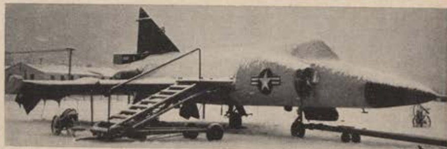
An F-102A undergoing Arctic testing at Ladd AFB. After a cold soaking that lasted twenty-four hours, the aircraft was flown, to prove fitness for Alaska.
