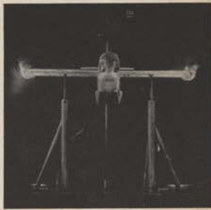
Bell's XV-3 convertiplane in NACA's Ames Laboratory during tunnel test.
