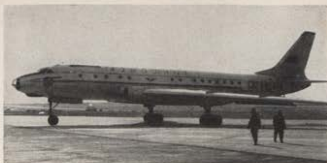
The TU-104 at Prague. Note chin radar and astrocompass dome. Craft cruises at 500 mph, has range of 1,900 miles.
