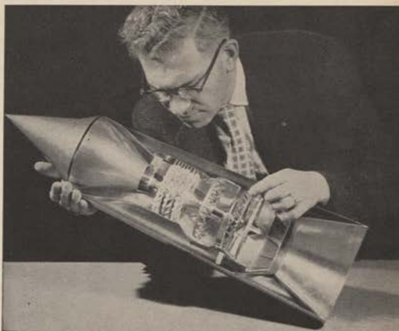
Model of theoretical 2,600-mph turbojet engine has only three compressor rows instead of the usual fifteen. The unit will be much more efficient than present equipment.
