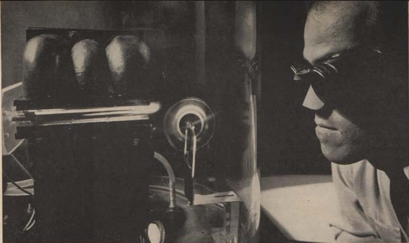
A miniature laboratory ion-propulsion model, operating at near-vacuum conditions, produces thrust which is detected by the small wheel behind the jet. Ion-propulsion units serving as low-thrust engines may be useful in space flight.
