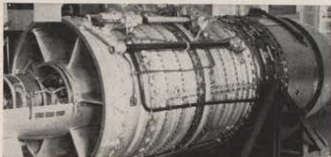
The AM-3 engine, photographed by the authors in Moscow Air Museum. The casing is split horizontally and radially. Bolt heads for stators appear through casing wall.
