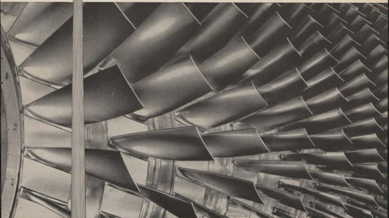
Rotor Blade Assembly of J-57 Engine which uses Eaton blades. The J-57 is the predecessor of the more powerful J-75.
