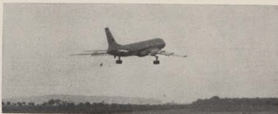
TU-104 took about 5,000 feet of runway on takeoff at Prague. Three-quarters of a mile out, it's no higher than this, and plane's wheels are still down.
