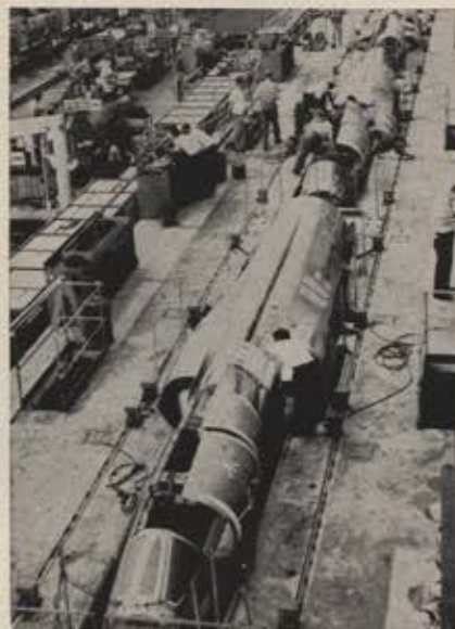
Lockheed F-104 fuselage assembly line at Burbank, Calif. After mating the fuselage sections in the area shown here, the entire fuselage is taken by truck to the company's Palmdale plant for final assembly and flight testing.
