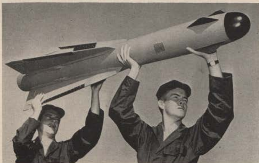
USAF's Falcon missile, a guided aircraft rocket, carries its own powerplant which drives it at supersonic speed. Airmen here ready it for a launching test.
