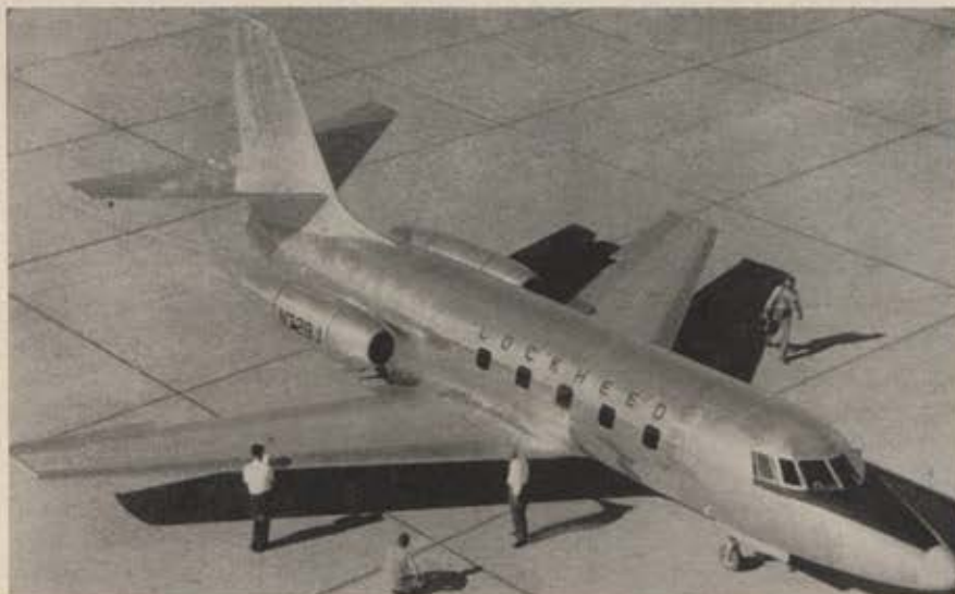
Lockheed Aircraft Corp. produced its new ten-passenger utility transport, the "JetStar," in thirty-four weeks from the day engineering started. Powered by two Bristol Orpheus jet engines attached to the rear of the fuselage, it can cruise at 500 mph at 40,000 feet. Engine location results in low sound levels in passenger compartment. They are easily accessible for ground maintenance.
