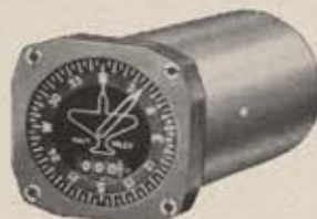
FLIGHT INDICATOR of this system displays ground track, required course, heading error, and distance to the destination.
