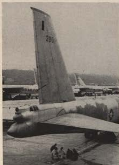
Vertical fin on Boeing B-52A has been shortened by six feet in test to improve production bombers. Effectiveness of cross-wind landing gear made smaller fin surface possible. Short fin reduces drag and increases range.
