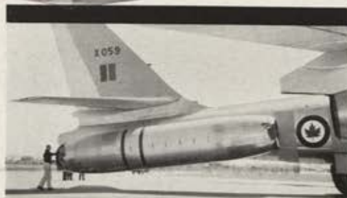
FLIGHT TESTING THE NEW IROQUOIS AT MALTON The supersonic Iroquois is carried in this specially designed pod at the rear of a B-47.
