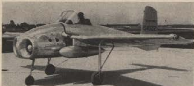
Bell X-14 (above) uses system of vanes controlling direction of thrust from engines to rise and land vertically while plane maintains horizontal attitude during flight.
