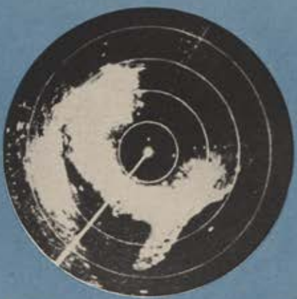
SEARCH: Gives pilot view for terrain clearance and sea search at ranges to 240 miles.
