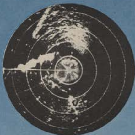
WEATHER WARNING: Shows pilot clear view of weather ahead up to 240 miles, enabling him to avoid thunderstorms, line squalls.
