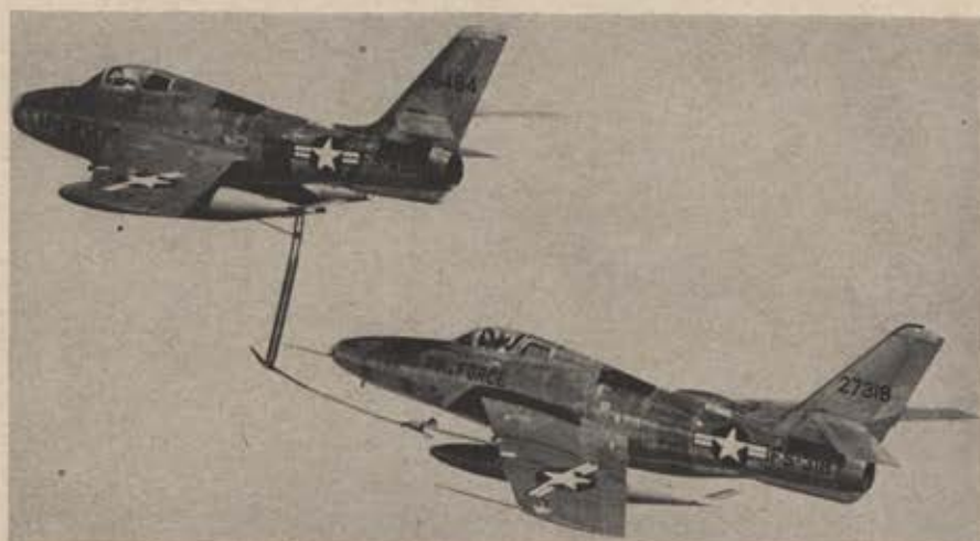
Republic Aviation's aerial refueling system converts fighters to tankers and back again in minutes. RF-84F Thunderflash (bottom) refuels from a F-84F.
