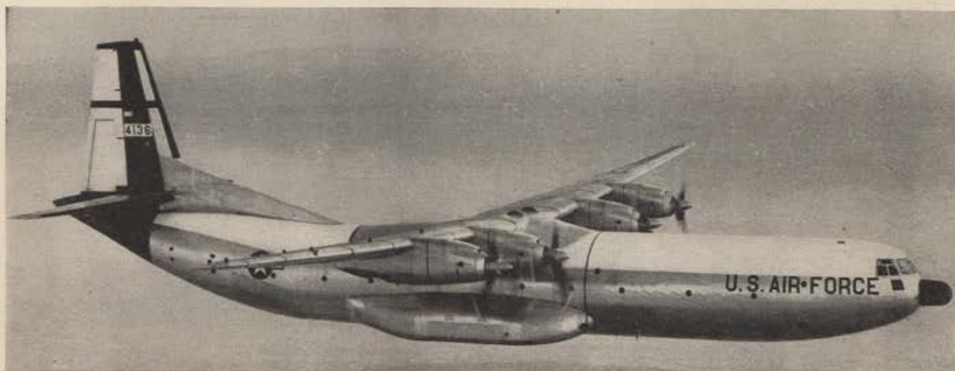
Now in MATS service out of Dover AFB, Del., is the giant new Douglas C-133 four-engine turboprop transport. The new carrier, which has a wingspan of 179 feet, eight inches, can carry payloads in excess of 3,000 miles. Production is in California.
