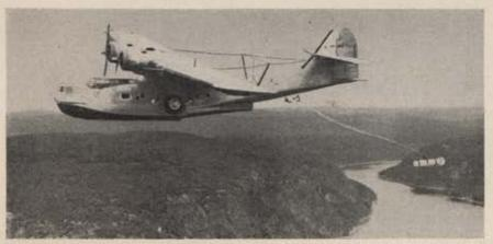
A Canso PBY flying laboratory tests mineral detection electronic equipment.
