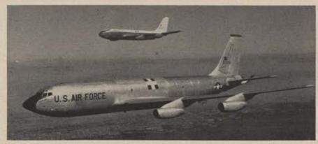
The first production model of the Stratotanker is paced in a test flight over Seattle by a Boeing 707, prototype of the commercial version of the KC-135.
