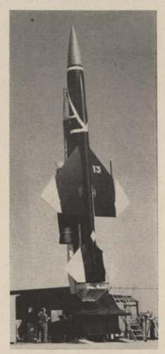
Boeing's Bomare is launched vertically by liquid fuel rocket motor. Two ramjet engines power the missile on its long-range flight toward the target.
