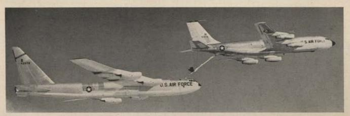
For the first time the tanker plane is in the same league with the bomber it refuels. Able to fly more than 550 mph and at altitudes above 42,000 feet, the KC-135 can completely replenish a B-52's tanks in less than half an hour.
