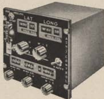
COMPUTER CONTROL feeds wind, variation, and destination data into the system. It displays present position, wind speed and direction, variation, and destination coordinates.
