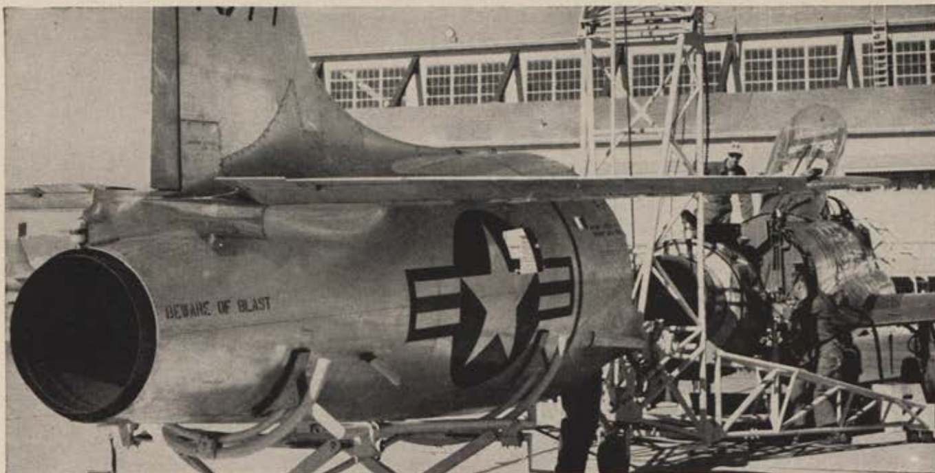
Laredo AFB crew replacing a J35 engine in a T33 trainer.
