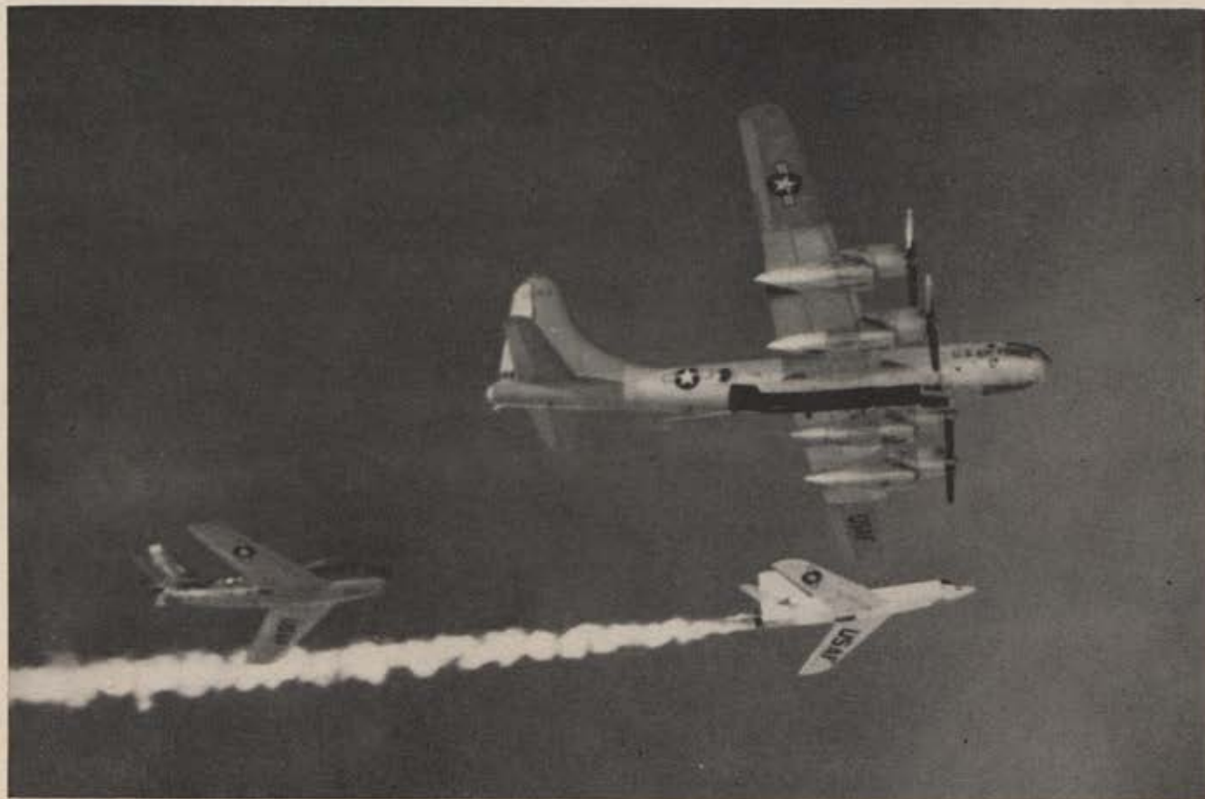
The X-2 began its test flights in August 1955. Here, in an early test, the X-2 is dropped from its B-50 "mother."
