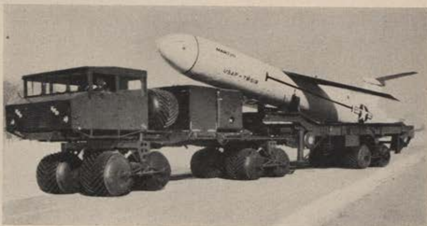
Multi-purpose "pillow-tire" Tera-cruzer with eight-wheel drive—built by Four Wheel Drive Auto Co.—and Goodyear Aircraft's Translauncher trailer are designed to blaze their own trail to off-road launching sites for Martin Matador.
