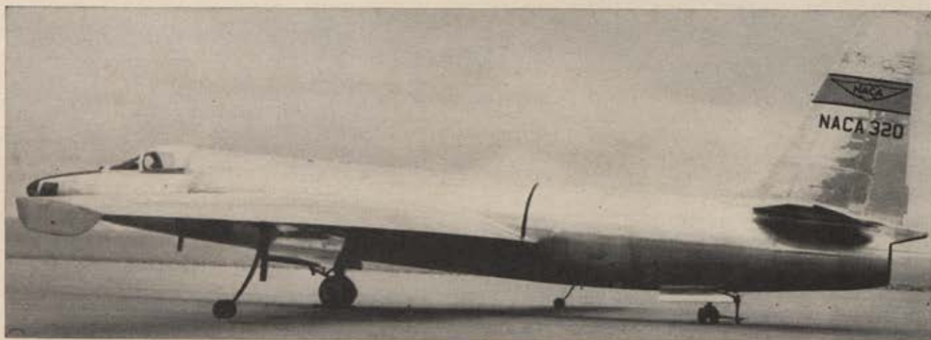
NACA uses Lockheed U-2 in research program into gust-meteorological conditions at altitudes of up to 55,000 feet.
