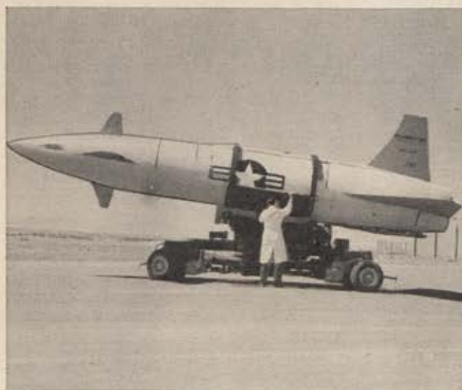
First photo of the Bell GAM-63 Rascal guided missile, a supersonic, rocket-powered, air-to-surface missile for AF use, shows Rascal with its ground handling equipment. The missile has been undergoing tests at Holloman AFB, N. M.
