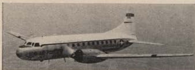
Test combination on the MATS Convair YC-131C includes Allison YT-56-A3 engines and Aeroproducts turbine propellers.
