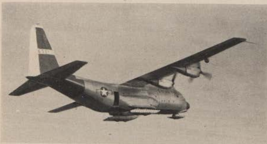
Lockheed C-130 on first flight with skis. In-flight behavior of the nineteen-foot skis was monitored by television mounted in pod under right outer wing.
