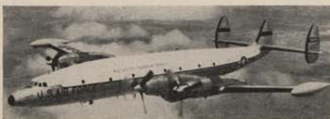
Lockheed Super Connie C-121C was fitted with Pratt & Whitney T-34-P6 engines, Hamilton Standard turbomatic props.
