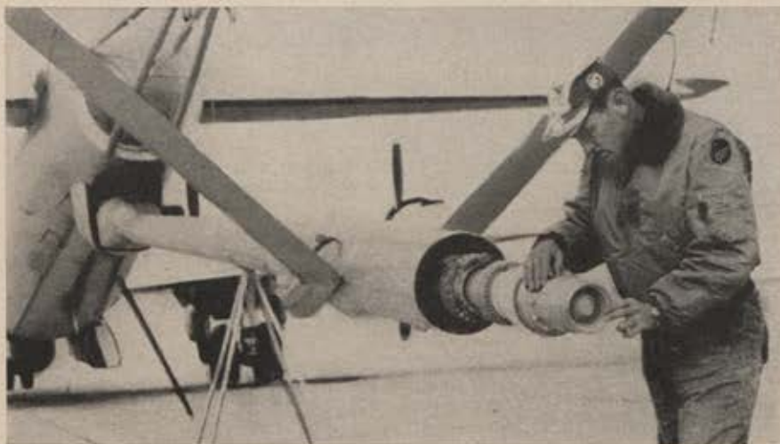
S/Sgt. Ray Lewis, a TAC KB-29 crewman, preflights his boom before take-off.
