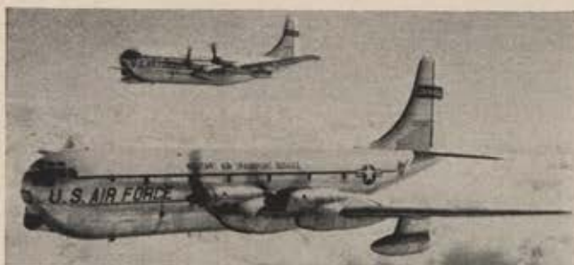
Pratt & Whitney T-34-P5 engines with Curtiss-Wright turboelectric props were used in MATS tests of Boeing YC-97Js.
