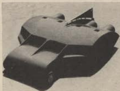
Hot rod! It's a bright red jet car (powered by four Allison J-33s), developed by All American Engineering Co. of Wilmington, Del., for the Navy, to test aircraft arresting gear. The driverless car roars down a test track at 200 mph, pushing a load equal to a twin-engine bomber, which is cut loose and slams into the arresting gear being tested.
