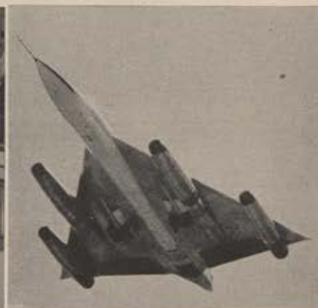
The B-58 Hustler is powered by four General Electric J-79 turbojets which thrust the delta-wing bomber along at supersonic speeds above 50,000 feet.
