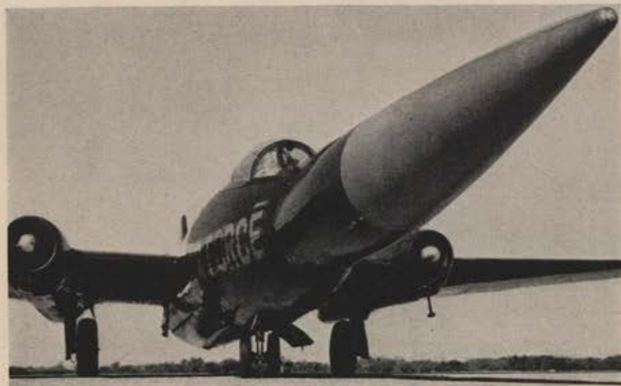
"Cyrano-Bomber" is a modified Martin B-57 Canberra jet bomber with a special nose cone which will flight test guidance systems for Boeing's Bomarc missile.
