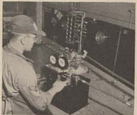
Under pressure test, this Aeroquip Hose Assembly withstands 4500 psi.
