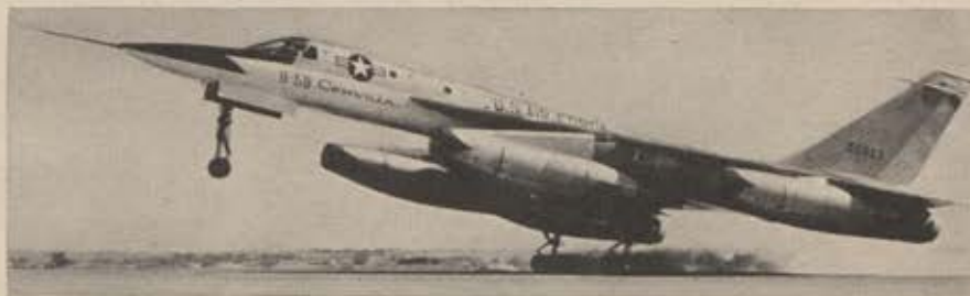
Convair's B-58 Hustler is America's first supersonic bomber. Its wing span is fifty-five feet, length ninety-five feet, and it carries a three-man crew.
