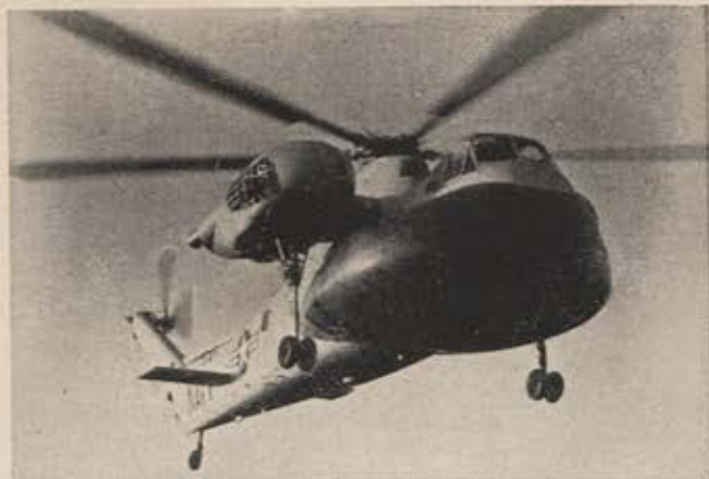
NEW RADAR HELICOPTER —Under development for the Navy by Sikorsky Aircraft is this HR2S-1W helicopter with radome accommodating search radar gear. It can extend radar coverage beyond the range of shipboard radar or land-based radar picket aircraft.
