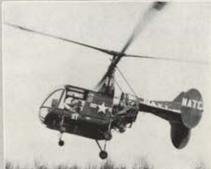
Kaman Aircraft and Lycoming scored a turborotor first when this Kaman HOK helicopter took to the air powered by Lycoming's XT-53, the first U.S. free-shaft gas turbine specifically designed as a helicopter power plant.
