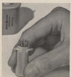
Latest addition to General Electric's line of hermetically sealed relays qualifies for severe-condition applications.
