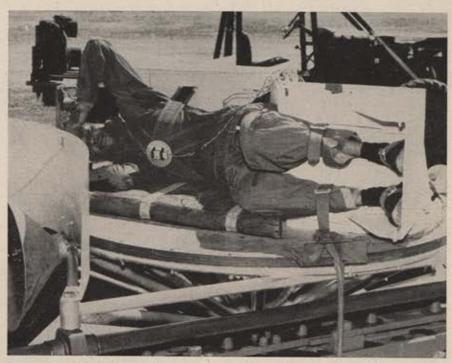
Subject on ARDC's "Daisy Track" (see text), can be rotated to different angles to determine the human tolerance of abrupt deceleration in various positions.
