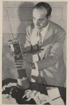
Radiosonde weather station dropped by planes over oceans and polar regions transmits weather data back to plane.
