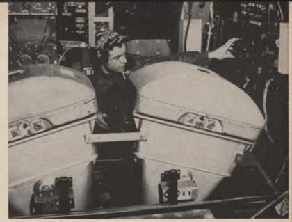
An operator between two huge aerial cameras in an RB-29 sets intervalometer that controls time between exposures.
