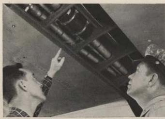
Mounted in each of the three refueling lines on the tanker, the General Electric in-flight refueling transmitter meters fuel to the receiving aircraft at pressures up to 480 pounds per square inch.
