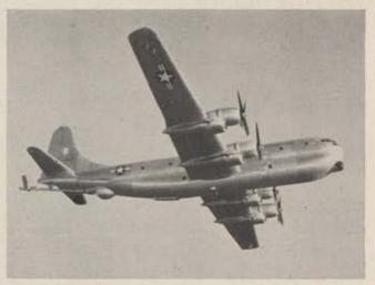
Boeing KC-97F, tanker version of the Stratofreighter. The boom, used for aerial refueling, is shown in retracted position. Boeing is now producing an all-jet tanker version of its 707 jetliner to make aerial refueling easier.
