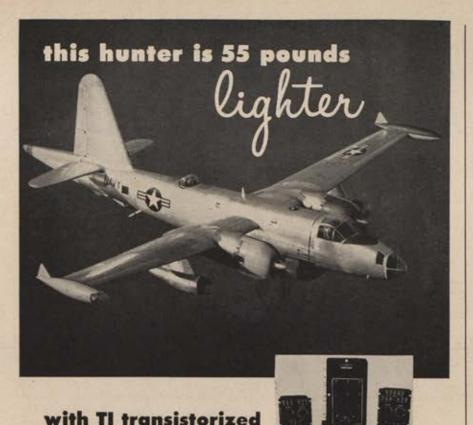
TI PRODUCTION ENGINEERING helped Lockheed trim 55 lb of dead load from the P2V-7 sub-hunting Neptune ... by transistorizing just one system - the 14-station intercom. In addition to saving weight, safety and reliability were increased while maintenance and power drain were reduced.
