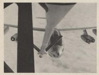
A real-life SAC B-47 prepares to take on fuel from a KC-97 tanker. The man who "lowers the boom" is known in AF circles as "Clancy." After the connection is made, fuel is pumped under great pressure through the boom.
