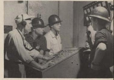
X405 ENGINE RUNS ARE CONTROLLED from blockhouse, adjacent to firing pit. Completely instrumented test cells record continuous performance data during close-to 150-second run.
