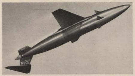
Radioplane's rocket-powered drone, designed for weapon systems evaluation and training at speeds of Mach 0.9 at 50,000 feet, has ten-minute flight endurance.
