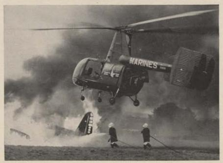
Fire-fighting helicopter, Kaman HOK-1, hovers over burning airplane, beating flames back with rotor downwash as two firemen approach to rescue the pilot.
