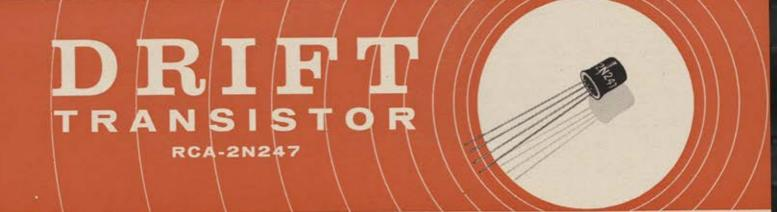
Designed to provide a "built-in" accelerating field in the base region that propels charge carriers from emitter to collector, RCA-2N247—a germanium p-n-p type transistor—begins a new era in transistor operation at radio frequencies extending from the lower frequencies well up into the short-wave bands.
