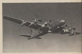
1945 Standard equipment on the Boeing B-50 included an advanced General Electric, remote-controlled armament sighting system.
