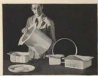
EASILY FORMED. These HK31A parts were drawn using production dies and processes for standard magnesium alloys. The parts retained a higher percentage of original properties than standard alloys.
