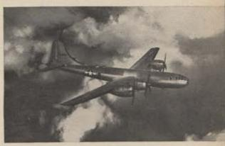
1942 Boeing B-29 Superfortress was defended by the first remote-control armament system including General Electric controls and turrets.
