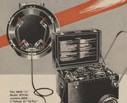
Two of the most important factors that affect jet engine life, efficiency, and safe operation are Exhaust Gas Temperature (EGT) and Engine Speed (RPM). Excess heat will reduce "bucket" life as much as 50% and low EGT materially reduces efficiency and thrust. Any of such conditions will make operation of the aircraft both costly and dangerous. The IETCAL Analyzer predetermines accuracy of the EGT and (interrelatedly) Tachometer systems and isolates errors if they exist.
