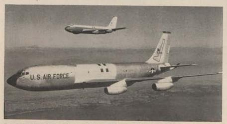
Boeing's KC-135 Stratotanker "City of Renton" (foreground), first production model of the jet tanker-transports being built for the Air Force's Strategic Air Command, is shown in formation with the Boeing 707 jet transport prototype on the initial flight of the KC-135, August 31. The new four-jet plane is one of a number ordered by the AF for aerial refueling of USAF jet bombers.
