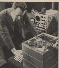
General Mills Pioneers Scientific Frontiers One of General Mills' numerous research projects involves the behavior of metals in space flight. Here a scientist determines the "sputtering" or disintegration rate of molybdenum at 200 miles above the earth. The metal is under fire from atoms moving at 25,000 m.p.h.
