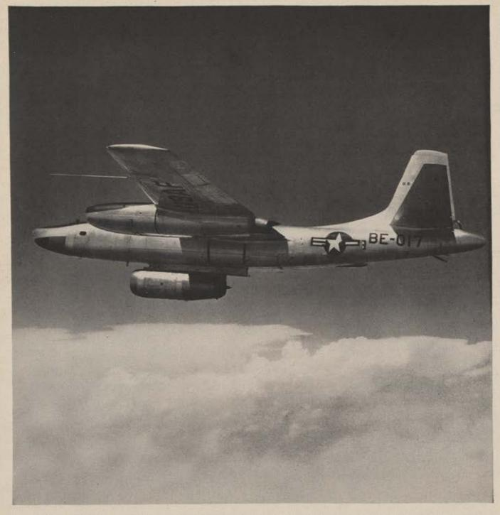
A J-75 TURBOJET ENGINE flies regularly beneath this special North American B-45 test-bed in its current exhaustive flight development program. The pod-mounted engine retracts into the bomb bay when not in operation. The J-75 has been announced as the engine for the Air Force Republic F-105 and the Navy Martin P6M.
