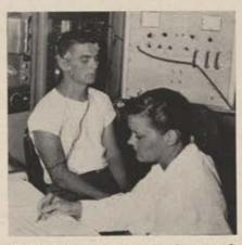
Period analyzer, a medical research instrument developed by the American Machine & Foundry Co., New York, will provide a faster and more accurate means of determining which men are best suited to stand the stresses of the jet age. It will measure physiological changes affecting brain waves.
