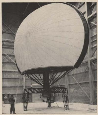
Mobile Paraballoon radar antenna can be disassembled and transported in standard trucks. Complete station can be assembled in two hours.
