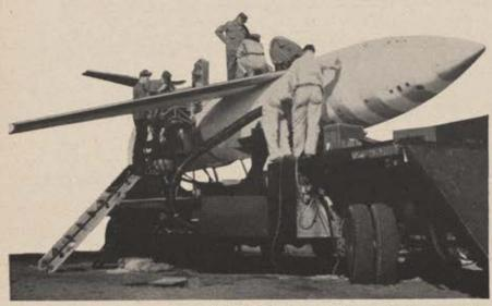
AF technicians prepare a Martin TM-61 Matador guided missile for launching at the Missile Test Center, Patrick AFB, Fla. Rocket propulsion unit is used to boost the Matador into the air, where its own jet engine takes over.
