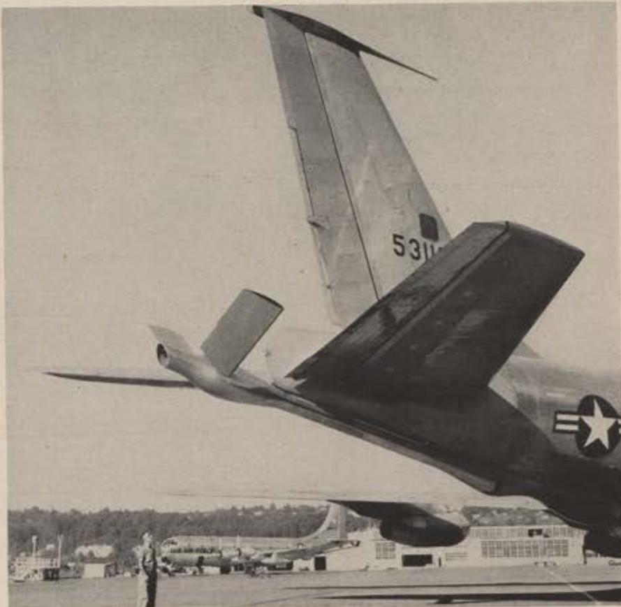
Boeing's first jet tanker, the KC-135, is equipped with the new streamlined flying boom and a new high-frequency antenna mounted on the vertical fin tip.
