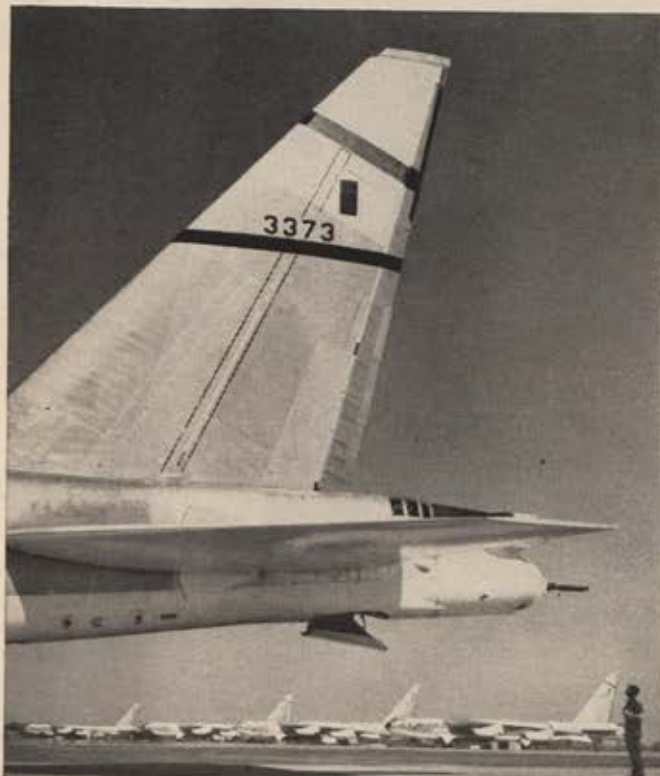
B-52 tail towers nearly five stories above ground. Rear tip of fuselage contains armament and fire controls.
