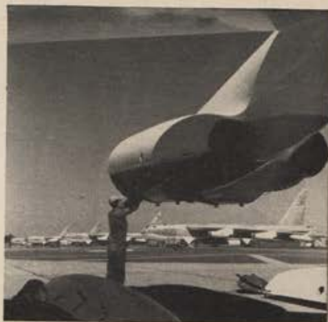
Two of the eight J57 jet engines that power the B-52. Suspended in pairs, the engines deliver more than 10,000 pounds of thrust each.
