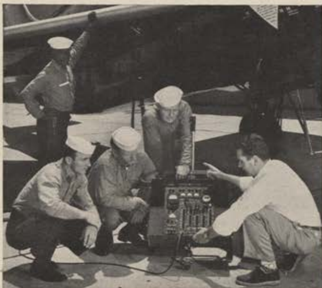
G-E SERVICE ENGINEER, Willie Jaques, demonstrates the autopilot line maintenance tester to Navy aviation specialists.
