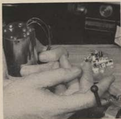
This small transmitter will send signals from the Vanguard space satellite.
