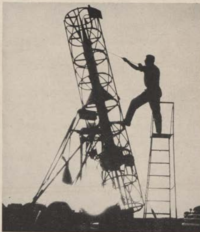
ARDC's Hypersonic Test Vehicle is readied for launching. It can reach speed of 5,000 mph two seconds after firing.
