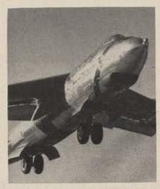
Lands big ones safely—BFG wheels, load-rated 60,000 lbs., give maximum strength with minimum weight on Boeing's B-47. What's more, this wheel stood up under test loads of 300,000 lbs.! B-47's dual wheel assemblies are equipped with B. F. Goodrich brakes.
