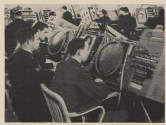
SAGE installations like this will enable the controller to handle a larger segment of the air battle at one time.
