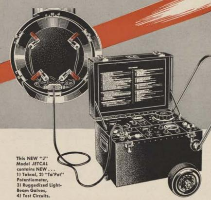
Two of the most important factors that affect jet engine life, efficiency, and safe operation are Exhaust Gas Temperature (EGT) and Engine Speed (RPM). Excess heat will reduce "bucket" life as much as 50% and low EGT materially reduces efficiency and thrust. Any of such conditions will make operation of the aircraft both costly and dangerous. The JETCAL Analyzer predetermines accuracy of the EGT and (interrelatedly) Tachometer systems and isolates errors if they exist.
