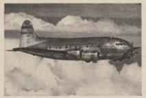
1939 'The 307, America's first four-engine, pressurized transport. First four-engine airliner in transcontinental service.
