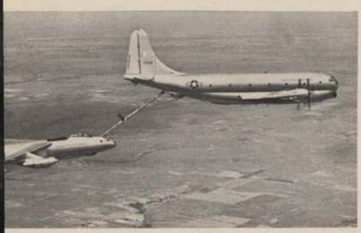
1947 B-47 six-engine Stratojet medium bomber, America's current frontline nuclear weapons carrier, being refueled in the air by a Boeing KC-97, standard aerial tanker of the Air Force.
