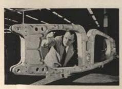
Left—a center section frame for a fighter-bomber, one of the largest single-piece forgings ever made, is examined by Nils Lou of the Republic Aviation Corp.
