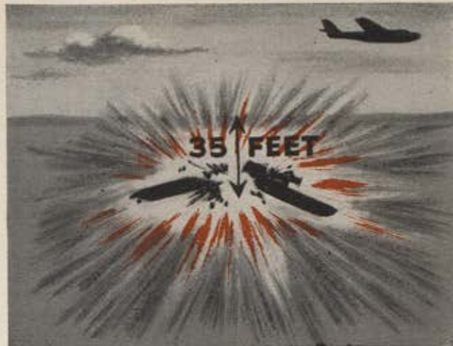
After careful analysis, it was found that the best exploding depth was thirty-five feet. The new setting increased the number of kills by so much that the Germans were led to believe that the British had doubled the explosive.
