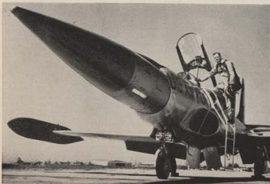
A modified Lockheed F-94 is used at the AF Missile Test Center, Fla., to test and evaluate missile components prior to their installation in test missiles.
