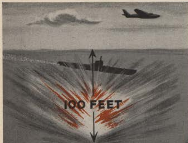
A good example of the value of operations research can be found in the experience of British anti-submarine operations early in World War II. Before a study was made, depth charges were set at 100 feet—with poor results.
