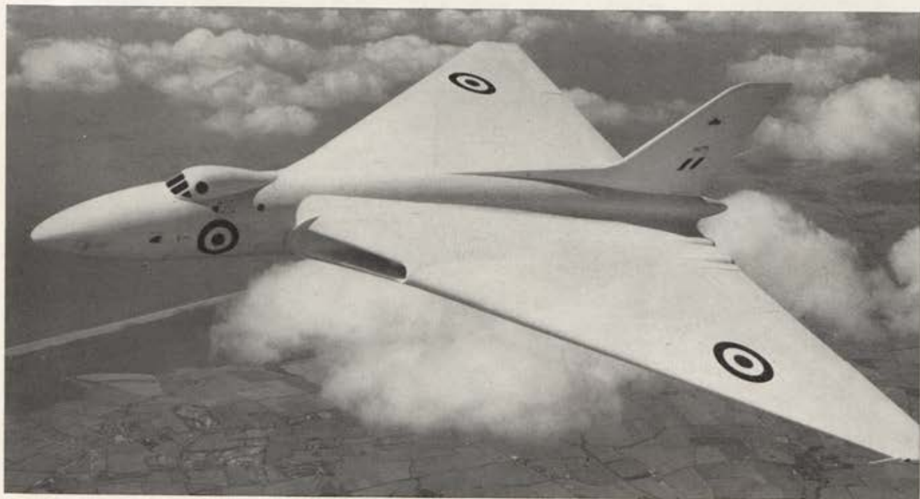
A. V. Roe's Vulcan has a delta wing with a span of 100 feet, is ninety feet long. It first flew in August 1952.
