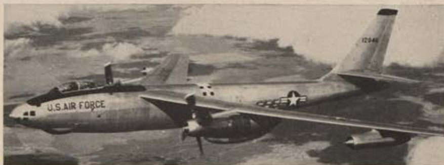
Boeing XB-47D Stratojet modified for the Air Force as a flying test bed for the Curtiss-Wright T-49 turboprop engine. The T-49s replace the usual inboard twin-jet engines. Propellers are Curtiss Electric, fifteen feet in diameter.
