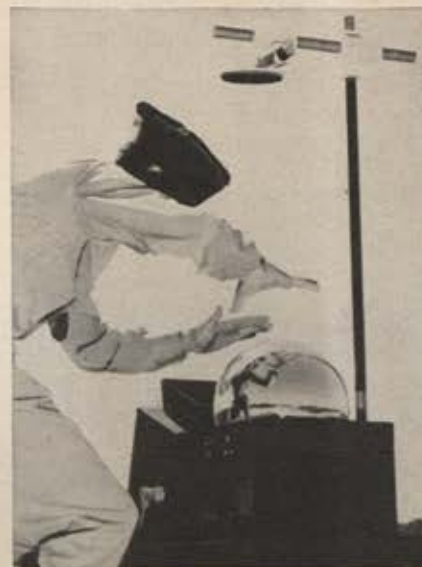
Crystal ball reflects the entire sky to a camera which takes a picture of the cloud coverage every fifteen minutes at AF Missile Test Center, Fla.
