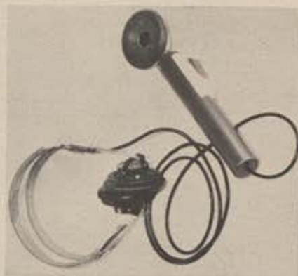
Transistorized intercom, designed by Goldak Co. for instructor-student use in noisy aircraft, is completely portable.
