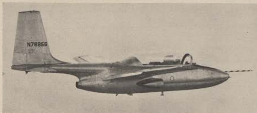
Temco's Model 51 primary jet trainer introduces the student to systems used in operational jet aircraft. It is equipped with ejection seats and a liquid oxygen system. The Continental YJ-60 engine can be changed in twenty minutes.
