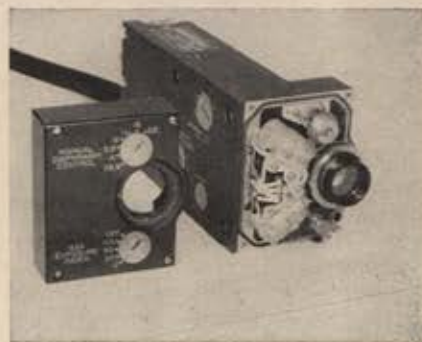
Miniature automatic exposure control mounted in Fairchild's new KB-5 gun camera can change aperture openings through six stops in 1.8 seconds.
