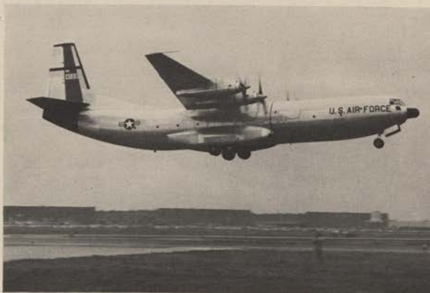
The Douglas C-133A turboprop transport—developed for the Military Air Transport Service—completes its first flight between Long Beach and Edwards AFB, Calif. It can haul 25 tons 3,500 nautical miles or 50 tons for 1,000 miles.
