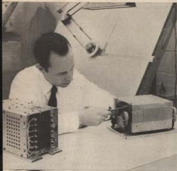
Main components of system include static voltage regulator and control panel.
