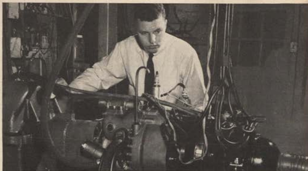
Alternator receives test. General Electric tested the complete F-101A electric system prior to first airplane installation.
