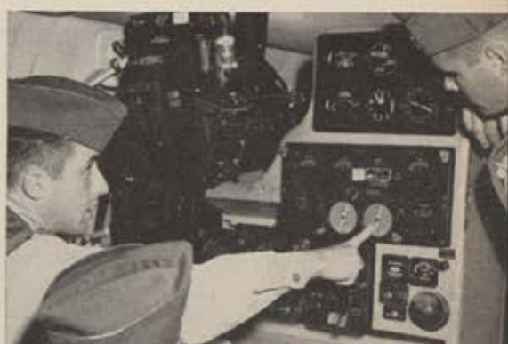
Q-24 radar in the T-29 does much of the computing for student navigators.
